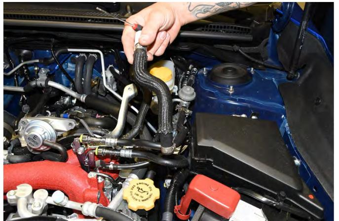
14. Using a ratchet and a 10mm socket, remove the (4) 10mm bolts that secure the throttle body to the intake manifold. If the throttle body is stuck, gently tap around the sides with a rubber mallet to break the throttle body free. Do not lose or damage the OEM Throttle-body gasket as it is reused.
