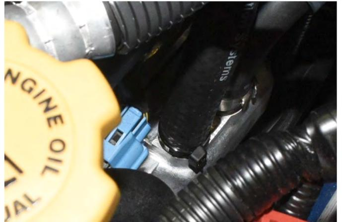
51. Trim the 1/2" hose to fit the center port on the AOS. Then install the hose onto the port. Install a zip tie on the hose at the center fire wall AC bracket as well as at the center AOS port. Trim off the excess.
