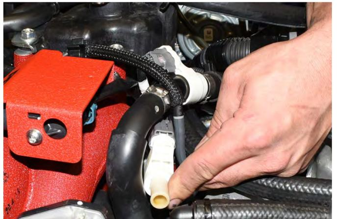
25. Remove the main engine harness from its mounting bracket located on the passenger side strut tower. Using a flat head screw driver pry the harness clip outwards and lift up as shown. In order to make room for the AOS carefully cut the OEM main wiring harness electrical tape at firewall as shown. (Harness is folded over itself under the tape). Refer to picture.
