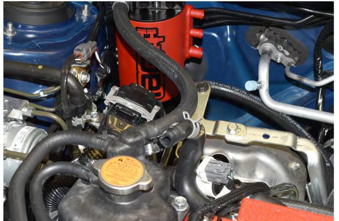
40. Locate the provided PCV hose as shown to the right. By hand, thread the side with the fitting into the upper AOS breather as shown. Once started use a 11/16 open end wrench to finish tightening the fitting.
