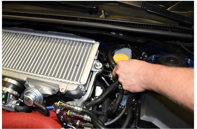
8. Using a 12mm socket, remove the intercooler mounting bolts on either side of the intercooler. In addition, remove the driver side intercooler bracket. It is held on by (2) 12mm bolts at the intake manifold.
