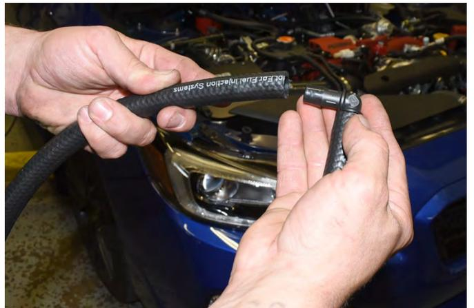
56. Route the 2" hose end to the passenger side crank case breather sensor and the remaining length of the 1/2" hose to the AOS upper left breather port. Trim the hose to fit as shown and secure the hose to the AOS and breather port using the supplied zip ties. Trim the excess off the ties when complete.
