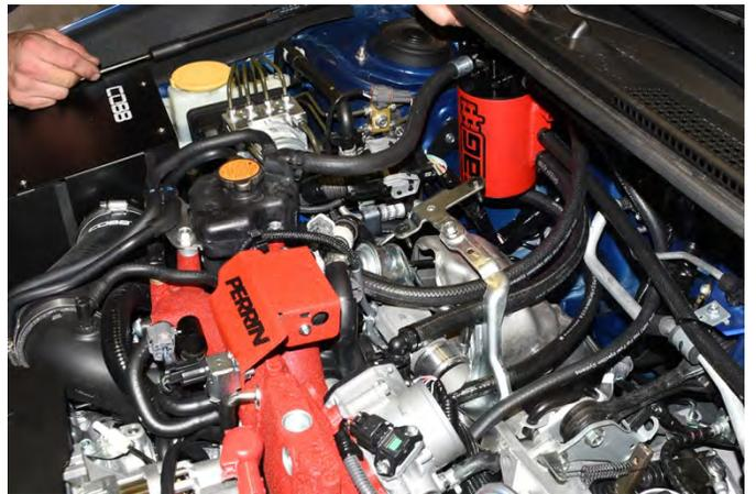
Next route the other side of the ½" hose under the intercooler bracket and alongside the 5/8" breather hose. The line will then lead up to the upper AOS side port. Make sure the line is free of kinks or any obstructions. Trim the line to fit and secure it with a zip tie trimming off the excess.
