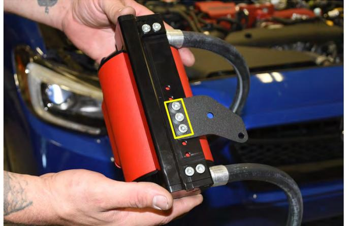
33. Install the AOS using the two holes on the strut tower shown in the picture. Guide the lower coolant hose underneath the main wire harness while installing the AOS. Start the upper M6x10mm bolt first then start the lower M6x10mm bolt. Once both bolts have been slightly threaded use a 10mm wrench to finish tightening them.
