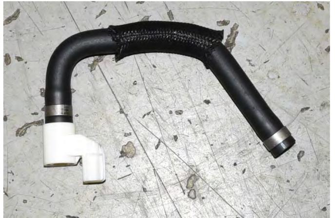
54. Remove the OEM hose from the crank case breather sensor and plug the white sensor back into the passenger side front electrical connector as shown.
