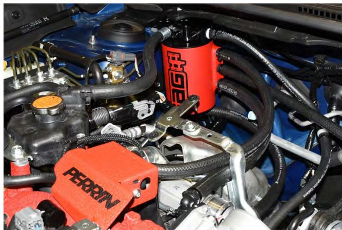
53. Locate the breather hard lines and remove the passenger side from crank case breather hose and sensor as shown.
