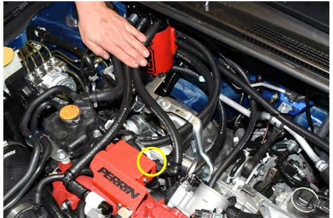
59. Reinstall the intercooler and bypass valve using the OEM hardware and gaskets. Reattach the negative battery terminal. Make sure to remove any fluid clamping pliers.
