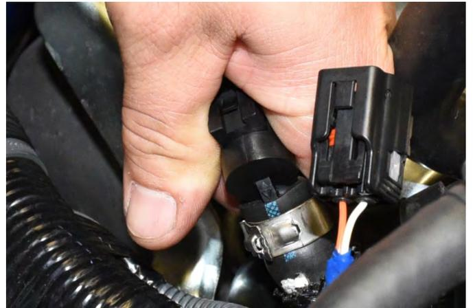
12. Locate the passenger side valve cover breather line (the one that is closest to the front of the car). Pull the hose off the valve cover port. Use a flat head screw driver if necessary to help free the hose off the port.
