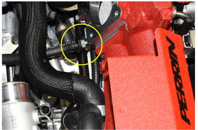
42. Re-install the throttle body to the intake manifold. Torque the (4) 10mm bolts to 6 <sup>lb</sup>/ft.
