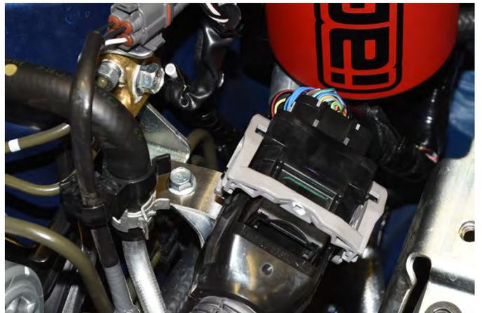
37. To minimize coolant loss, pinch off the lower coolant hose that connects the turbo to the cylinder head using hose clamping pliers.
