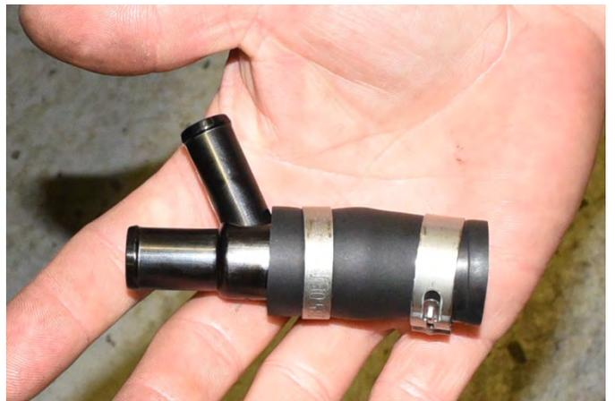
Drain fitting installed into the OEM  $\frac{3}{4}$ " hose
