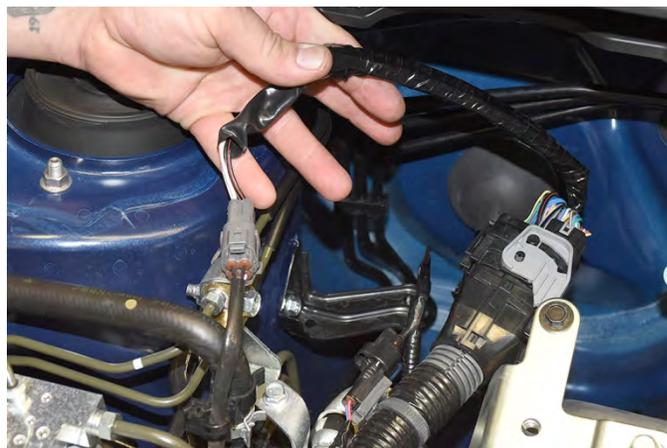
27. Remove main wiring harness bracket using 10mm socket and ratchet, it is held on by (1) 10mm bolt located on the passenger side strut tower.
