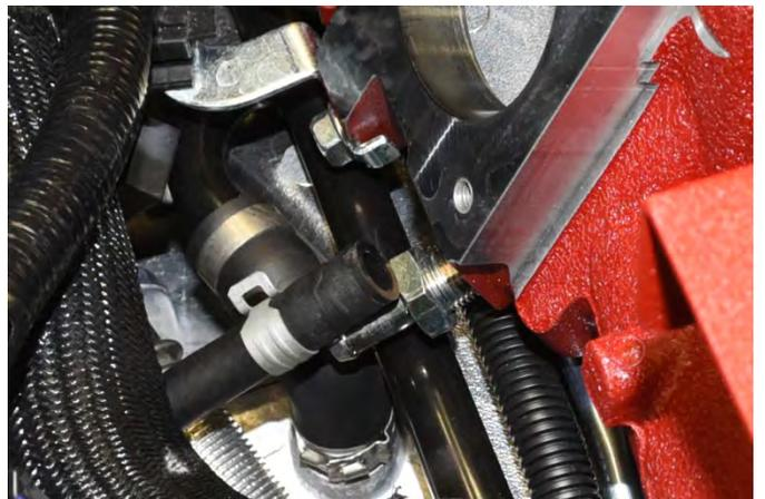
16. Next unplug the Passenger side Crankcase Ventilation Sensor that is located behind the intake manifold and in front of the turbo by pressing the gray clip in and pulling outwards.
