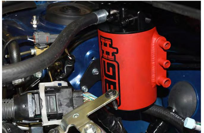
34. Use a 10mm socket and ratchet to remove the (1) 10mm bolt from the power steering line bracket located on the passenger side strut tower.
