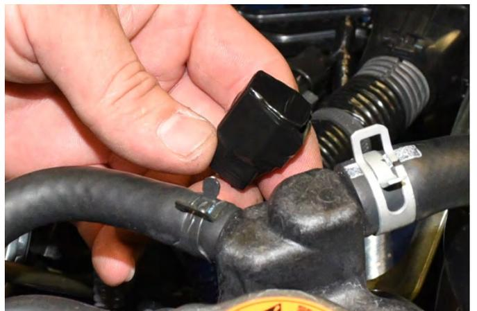
23. Locate the PCV assembly with the Crankcase Ventilation Sensor that was removed from the vehicle. Remove the (White) Crankcase Ventilation sensor from the hose.
