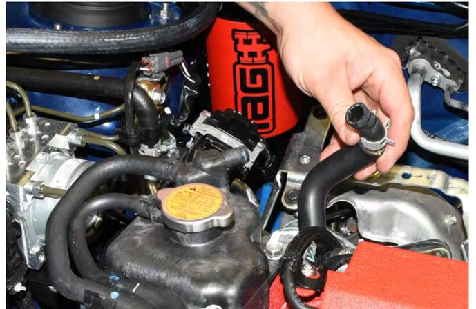
39. The IAG AOS upper coolant line will attach to the OEM coolant expansion tank. Trim the upper AOS coolant line to the correct length making sure when the line is routed there are not any kinks or obstructions. Once cut, using pliers pinch and slide the supplied pinch clamp onto the AOS coolant line. Then slide hose over the expansion tank port barb and secure the line with the clamp.
