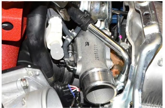
46. Secure the passenger side lower AOS coolant hose to the wiring loom bracket using a supplied zip tie. Trim off the excess using snips or scissors.
