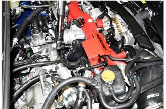
43. Locate the AOS lower coolant hose. The hose should be routed under the main harness and lead to the upper coolant hard pipe on the turbocharger. Trim the line to fit onto the upper coolant turbocharger hard pipe.
