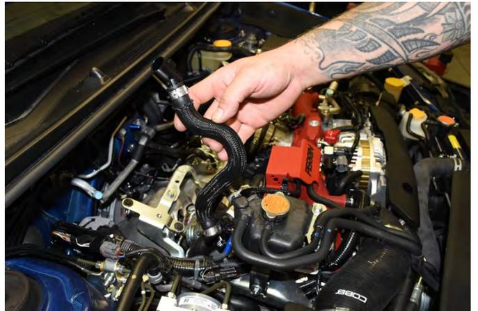
13. Repeat the process on the driver side forward most valve cover breather hose. Remove the driver side hose from the engine bay.
