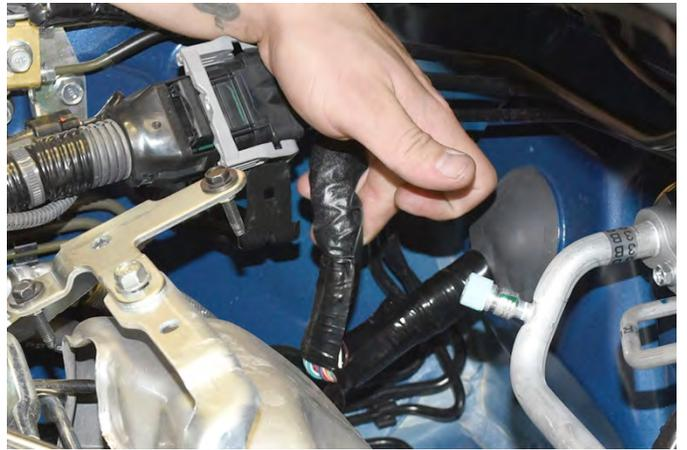
Main wiring harness shown after cutting tape
