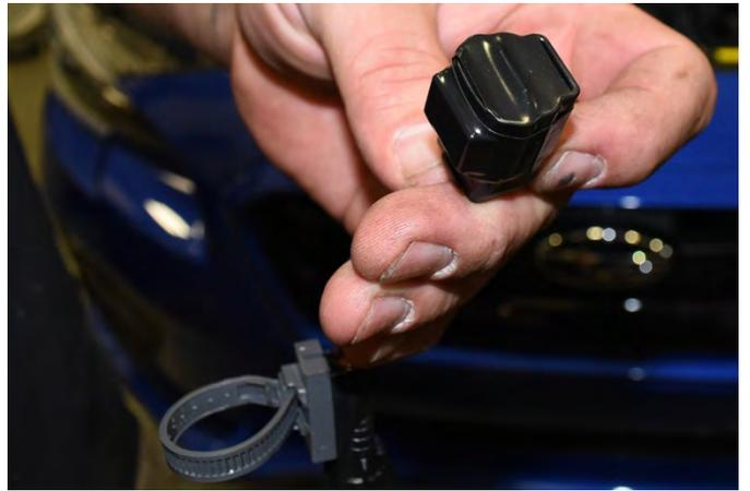
21. Reinstall the mini Crankcase Ventilation Sensor harness onto driver side hose as shown by reusing the OEM zip tie. Then plug the electrical connector back into mini harness.
