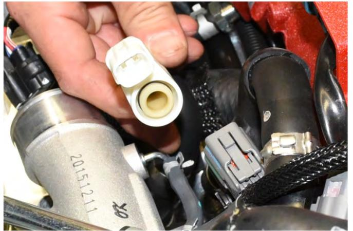
17. Remove the PCV valve assembly with the Crankcase Ventilation Sensor from the engine. It may come out with the  $\frac{3}{4}$ " drain hose. If the OEM drain hose is in good condition you will reuse it. We have supplied you with a new drain hose if the OEM unit is worn or damaged.
