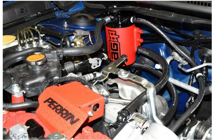
50. Locate the 1/2" breather line included in the AOS kit. Route one side of the line to the driver side most forward valve cover breather port. The line should pass above the AC line and over top the fuel injector cover bracket until it meets the valve cover port. Slide the hose onto the port and secure it with a zip tie.
