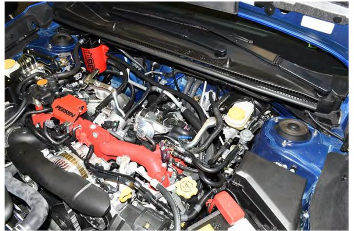
52. Using the remaining length of 1/2" hose, route it between the main harness and over top the injector cover bracket. Finally slide it onto the passenger side valve cover breather port and secure it with a zip tie and trim the excess off.
