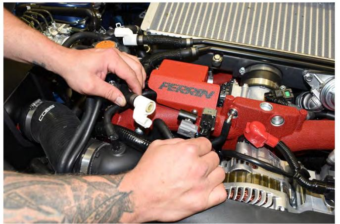
5. Using a 12mm socket, remove the (x2) 12mm bolts that hold the hard breather lines to the intercooler. Then remove the assembly from the vehicle.
