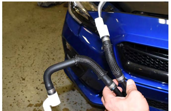
22. Remove the jumper from the white portion of the passenger side Crankcase Ventilation Sensor using needle nose pliers. Pull outwards from sensor until it is free. Then insert the jumper into the passenger side connector harness as shown. Tape the connector end with electrical tape to prevent exposure to the elements and tuck it out of the way.
