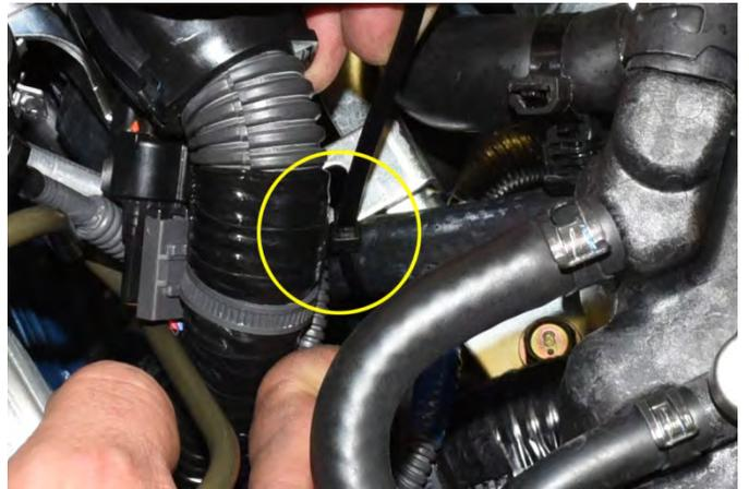
47. Locate the AOS oil drain line. The line will route over the transmission, thru the turbo support bracket and finally lead to the 1/2" port on the plastic drain fitting located on the engine block. The hose is supplied long to allow for various turbochargers, intercoolers and downpipes. Make sure when trimming the length that the hose is free of heat sources and the line is not kinked. Once the hose is in place install a zip tie to secure the hose and trim the excess.
