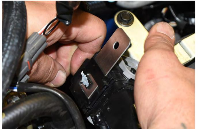
36. Next install the harness relocation bracket into the same location (power steering line bracket) using the same 10mm bolt. Do not completely tighten the bolt yet. Adjust the position of the main harness for clearance and fitment. Then finish tightening the 10mm bolt. Finally press down on the harness and slightly bend the bracket downwards as shown.
