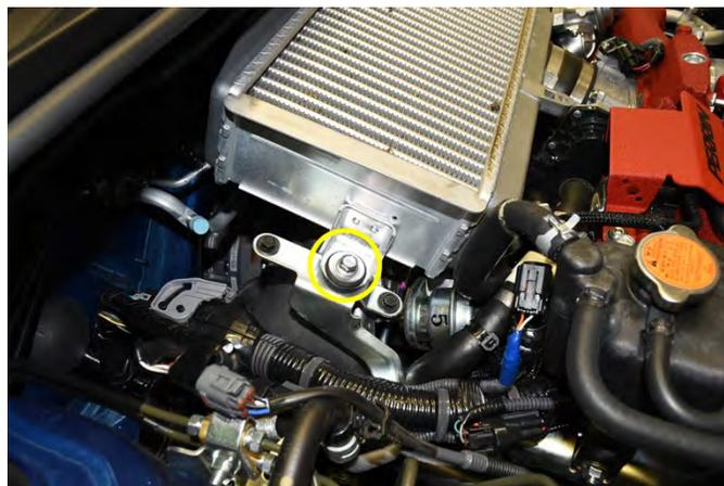
9. Using a flat head screw driver or 8mm nut driver, loosen the hose clamp at the intercooler outlet silicone coupler. Then loosen the hose clamp at the intercooler inlet.
