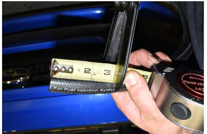
48. Locate the 5/8" breather hose and the plastic 90° fitting included with the AOS kit. Cut 3" off the breather hose. Slide the 3" length of breather hose onto one side of the 90° fitting, then slide the remaining length of 5/8" hose on the other side of the fitting. Zip tie the hoses on to the 90° fitting and trim off the excess.
