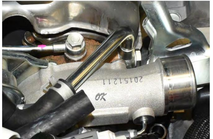
44. Using pinch pliers slide the OEM clamp down the OE upper turbo coolant line. Next slide the new supplied pinch clamp onto the lower IAG AOS coolant line at the turbo.
