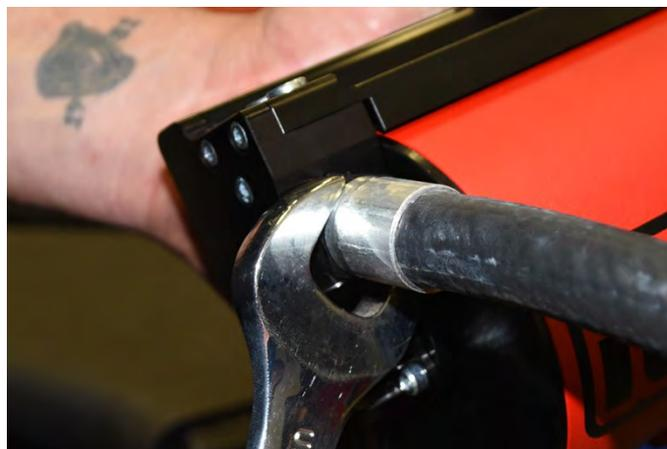
31. Install the 1/2" drain hose onto the AOS drain port fitting. Secure with a zip tie and trim the excess off.
