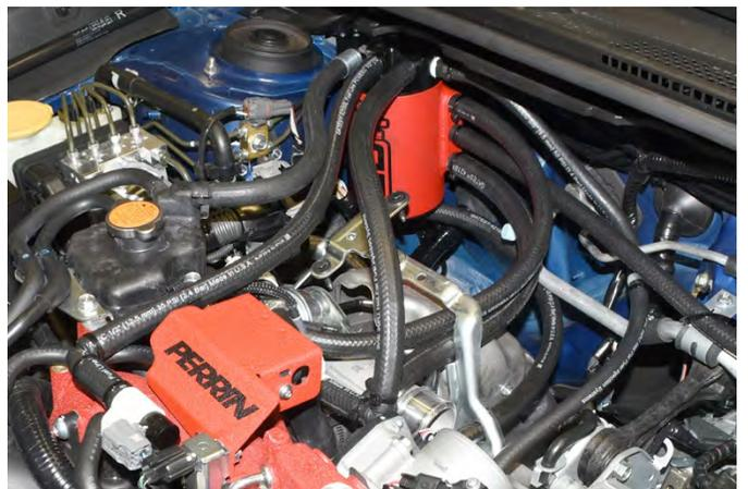
58. Route the 2" hose end to the passenger side rear crank case breather sensor and the remaining length of the 1/2" hose to the AOS upper right breather port. Trim the hose to fit as shown and secure the hose to the AOS and breather port using the supplied zip ties. Trim the excess off the ties when complete.
