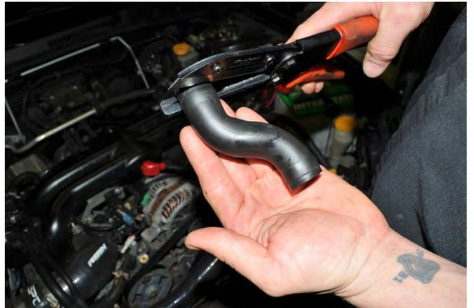
13.c (Early Model) Install the plastic “Y” fitting into the hose and secure it with original clamps. Install the drain hose assembly back onto the engine.
