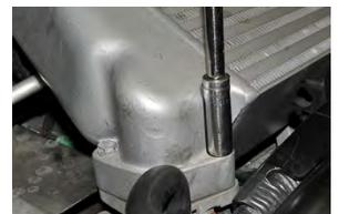
5. Using a flat head screw driver, loosen the hose clamp at the intercooler outlet silicone coupler.
