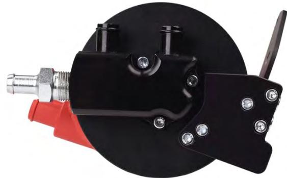
19. Next install the (2) AOS coolant lines onto the AOS (Lines come pre-assembled). Make sure the o-rings are lubricated (WD-40 / Silicone Lube) before threading them in by hand. Then tighten them using a  $\frac{7}{8}$ " open end wrench.
