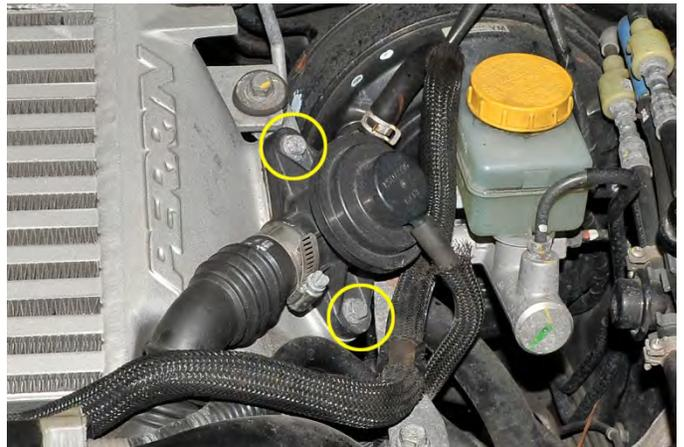
4. Using a 12mm socket, extension and ratchet remove the (3) 12mm bolts that secure the intercooler.
