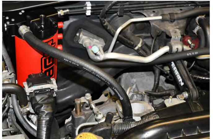
30. Locate the AOS lower coolant hose. The hose should be routed under the main harness and lead to the coolant expansion tank. Trim the AOS hose to fit onto the upper coolant expansion tank port. Make sure the hose is free of kinks or obstructions. Slide the new supplied pinch clamp onto it using pliers.
