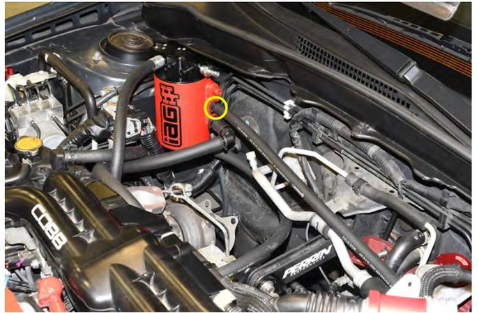
37. Using the remaining length of ½" hose, route the hose between the main harness and over top of the fuel injector cover bracket. Finally slide it onto the passenger side valve cover breather port and secure it with a zip tie and trim the excess off.
