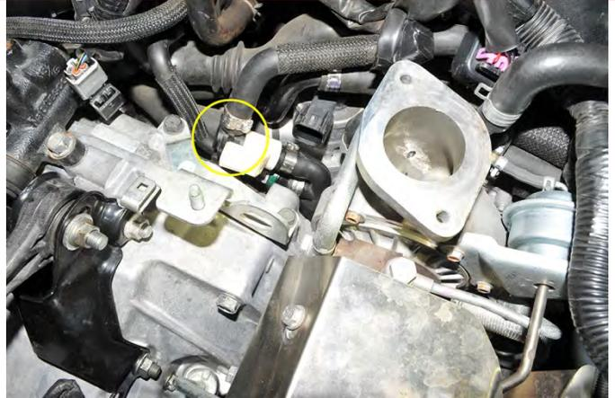
14.b Late Models: Remove the clamp that holds the hose to the PCV valve using a small flat head screw driver. Then remove the hose from the PCV valve.
