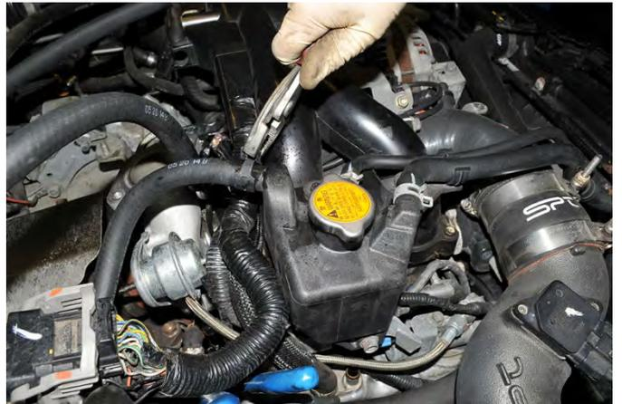
31. Remove the hose clamping pliers from the turbocharger coolant drain line.
