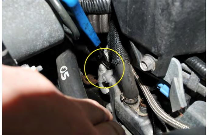
26. The upper IAG AOS coolant hose will attach to the OEM coolant hardline on the turbo. Trim the upper AOS coolant line to the correct length making sure when the line is routed there are not any kinks or obstructions. Once cut, using pliers pinch and slide the supplied pinch clamp onto the AOS coolant hose.
