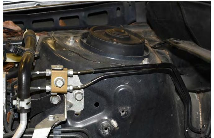
23. Locate the two mounting holes indicated on the picture to the right. Using one of the included M6x12mm bolts, thread the bolt through each hole to remove any foreign media. Remove the hardware after cleaning the threads.
