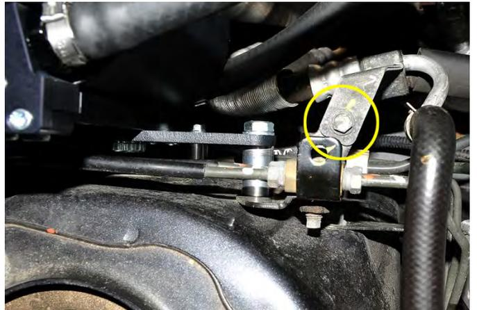
Next install the supplied harness relocation bracket using the same 10mm bolt. Do not completely tighten the bolt yet. Slide the harness onto the relocation bracket until it clips into place. Then adjust the position of the main harness for clearance and fitment. Then finish tightening the 10mm bolt.
