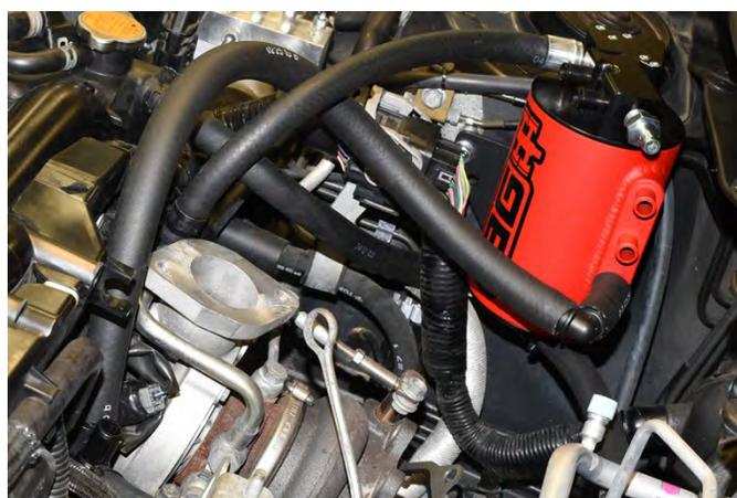
34.b. (LARGE TMIC) Slide the long  $\frac{5}{8}$ " breather hose onto the other side of the 90° fitting. Route the breather line to the  $\frac{5}{8}$ " port on the AOS can. The line should route by the intake manifold as shown. Trim the line to fit. Leave enough room so the line is free of obstructions and not kinked. Secure all the hose connections with zip ties and trim the excess off.
