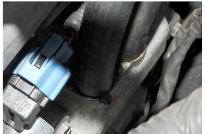
36. Route the remaining length of hose following the AC line to the passenger side where the AOS is located. Trim the hose to fit the center port on the AOS. Make sure the line is free of kinks and any obstructions; then install the hose onto the port and secure it with a zip tie.
