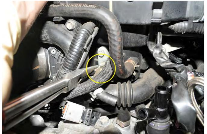
16. Remove the main engine harness from its mounting bracket located on the passenger side strut tower. Using a flat head screw driver pry the harness-clip outwards and lift up. Remove the plastic clamp holding the main harness to the strut tower. Refer to picture.
