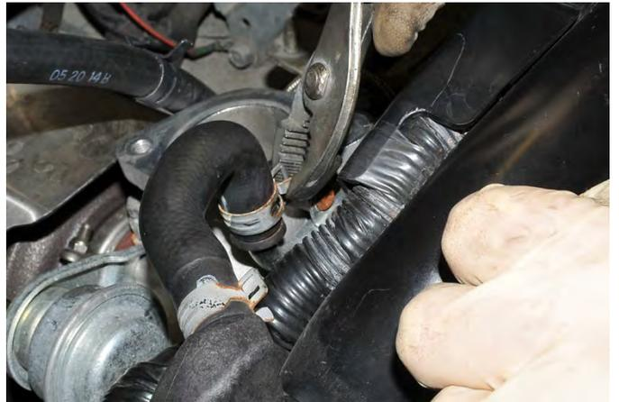
28. Next remove the OEM clamp off the coolant expansion tank. Remove the OEM hose as shown.
