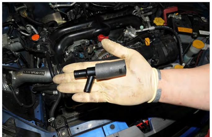
15. Remove the small pinch clamp and hose from the PCV vacuum nipple located by the throttle body on the intake manifold using needle nose pliers. Place the hose to the side it will not be used later.
