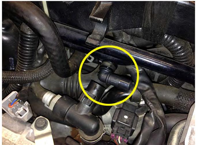
9. b Remove the jumper from the white portion of crankcase blow-by sensor using needle nose pliers. Pull outwards from sensor until it is free. Then insert the jumper into the gray blow-by sensor connector using needle nose pliers. Tape the connector end with electrical tape to prevent exposure to the elements and tuck it out of the way.
