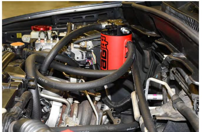
38. Locate the  $\frac{1}{2}$ " 90 degree fitting that you installed at the blow by sensor location (Step 9.a). Using the supplied 37" length of  $\frac{1}{2}$ " hose, attach one end onto the 90 degree fitting and route the other end to the right side upper breather port of the AOS as shown. Trim the hose to fit. \* Note the length of hose should be approximately 19". Secure each end of the hose with zip ties and trim off the excess.
