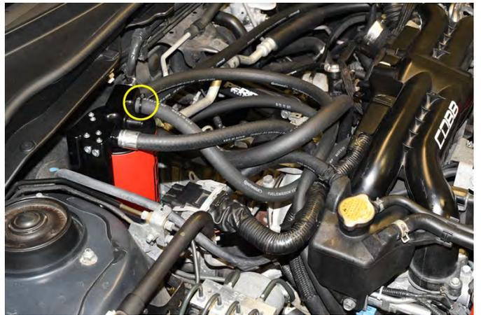
39. Locate the  $\frac{1}{2}$ " –  $\frac{3}{8}$ " adapter union installed at (Step 11). Install the remaining length of  $\frac{1}{2}$ " hose onto the barbed end of the fitting then route the hose to the left upper breather fitting on the AOS as shown. Trim off the excess length of hose (if any). \*The line should be approximately 15" in length. Secure the hose with zip ties and trim off the excess.
