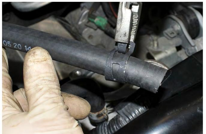
27. Using pliers remove the OEM clamp off the turbocharger's upper coolant hardline.
