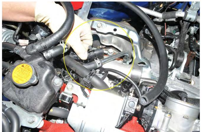
Remove the upper OEM coolant line pinch clamp and pull the OEM line off the turbocharger. Remove the OEM line from the vehicle.
