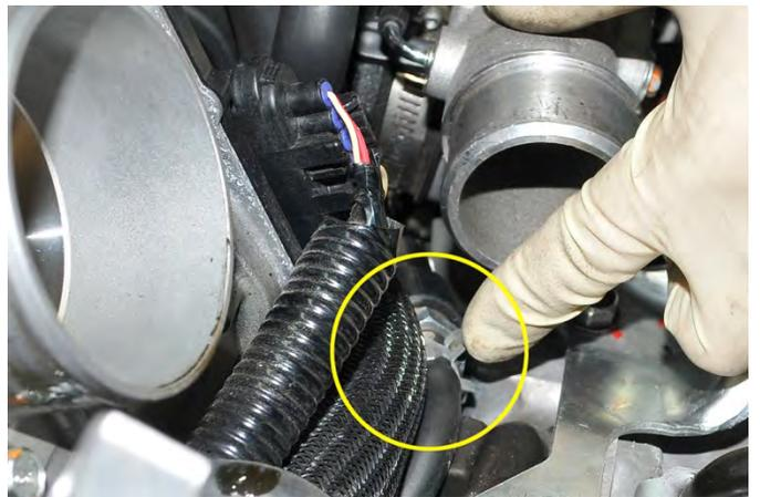
11. Remove the PCV valve assembly from the engine. It may come out with the  $\frac{3}{4}$ " drain hose. If the OEM drain hose is in good condition you will reuse it. We have supplied you with a new drain hose if the OEM unit is worn or damaged.
