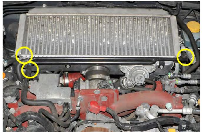
4. Using a 12mm socket, remove the intercooler mounting bolts on either side of the intercooler. In addition, remove the driver side intercooler bracket. It is held on by (2) 12mm bolts at the intake manifold.
