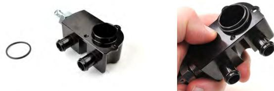
24. Clock the upper breather fitting so that it matches the picture. Locate the (3) supplied 4mm x 8 allen bolts and using a 3mm allen wrench thread the bolts through the breather fitting into the AOS and secure the port fitting.
