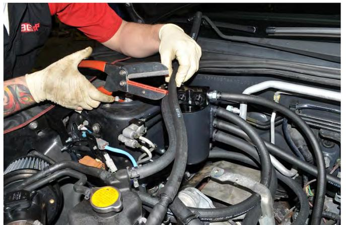
39. Locate the remaining  $\frac{1}{2}$ " hose supplied with the kit. Cut 2" off and insert it onto the supplied  $\frac{1}{2}$ " 90° degree plastic fitting. Then install the  $\frac{1}{2}$ " hose and 90 onto the white portion of the blow-by sensor.
