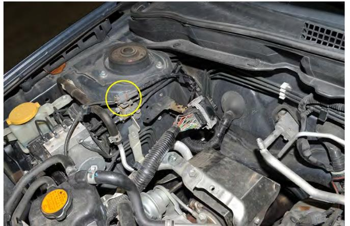
18. Remove main wiring harness bracket using a 10mm socket and ratchet, it is held on by (2) 10mm bolt located on the passenger side strut tower.
