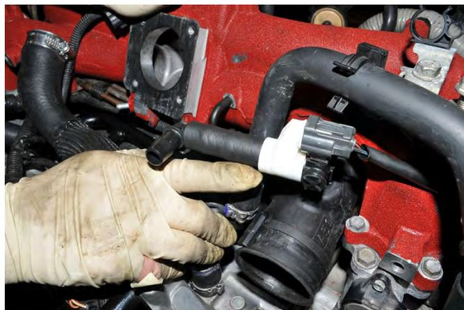
40. Install the remaining length of  $\frac{1}{2}$ " hose onto the plastic 90° fitting. Then route the remaining portion to the port on the AOS breather. Trim the excess and secure all the connections with zip ties.
