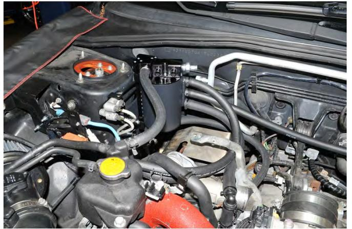
37. Route the 3/8" hose from the PCV nipple under the throttle body to the PCV located at the top breather port of the AOS. Keep the line as low as possible next to the transmission housing. Trim the hose to fit and secure with a zip tie. Trim excess off the zip tie.
