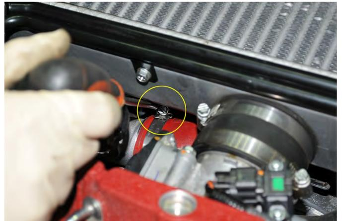
7. Using a flat head screw driver, loosen the hose clamp at the intercooler outlet silicone coupler.
