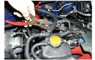
30. Locate the AOS lower coolant hose. The hose should be routed under the main harness and lead to the upper coolant hose on the turbocharger. Trim the line to fit onto the upper coolant turbocharger hard pipe. Slide the new supplied pinch clamp onto it using pliers.
