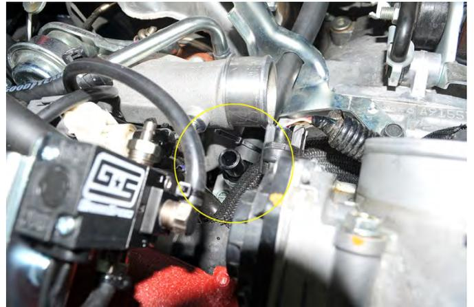
32. Locate the 5/8" breather hose and the plastic 90° fitting included with the AOS kit. Cut 3" off the breather hose. Slide the 3" length of breather hose onto one side of the 90° fitting, then slide the other side of the 3" breather hose onto the 5/8" port on the plastic drain fitting.
