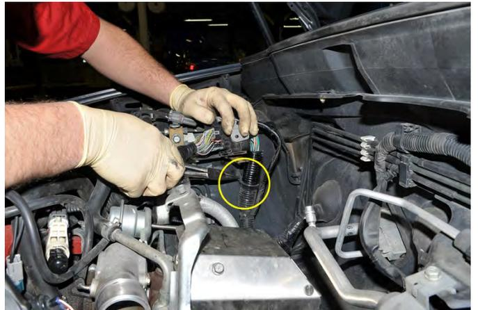
Unplug the primary O2 sensor and pull it free from the bracket to make space for the AOS install.
