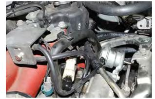
Finally using a supplied zip tie secure the line to the power steering bracket as shown. ***\*If done correctly minimal coolant should be lost. If substantial coolant is lost, bleeding the coolant system is required to avoid overheating.***
