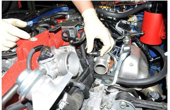
33. Slide the long 5/8" breather hose onto the other side of the 90° fitting. Route the breather line to the 5/8" port on the AOS can. The line should route over top of the heat shield and under the intercooler bracket. Trim the line to fit. Leave enough room so the line is free of obstructions and not kinked. Secure all the hose connections with zip ties and trim the excess off.
