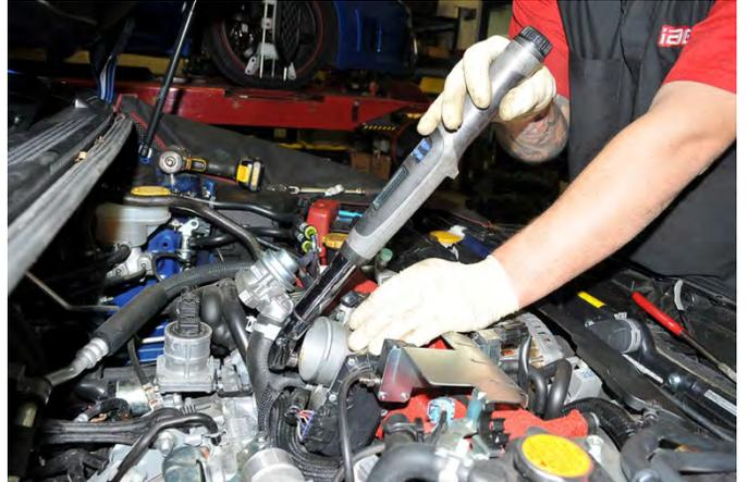
17. Remove the main engine harness from its mounting bracket located on the passenger side strut tower. Using a flat head screw driver pry the harness clip outwards and lift up as shown.
