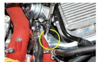
5. Using a 12mm socket, remove the (2) 12mm bolts that hold the blow off valve (BOV) to the intercooler. You can leave the BOV where it sits. Be careful not to lose or damage the gasket.
