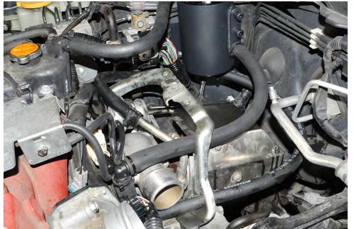
34. Locate the ½" breather line included in the AOS kit. Route one side of the line to the driver side most forward valve cover breather port. The line should pass inside the AC line and over top the fuel injector cover bracket until it meets the valve cover port. Slide the hose onto the port and secure it with a zip tie.
