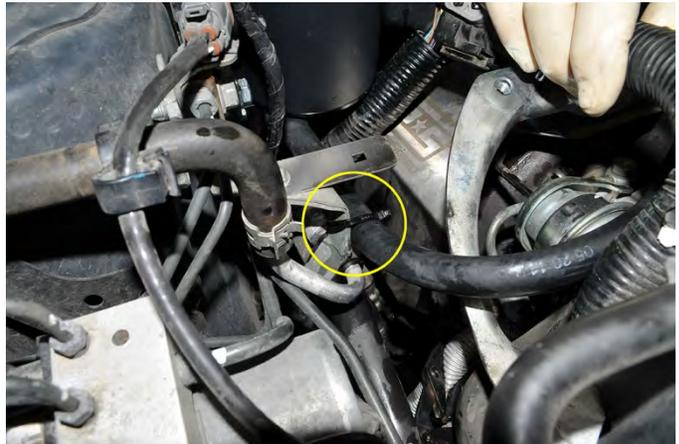
31. Locate the AOS oil drain line. The line will route over the transmission, thru the intercooler support bracket and finally lead to the 1/2" port on the plastic drain fitting located on the engine block. The hose is supplied long to allow for various turbochargers, intercoolers and downpipes. Make sure when trimming the length that the hose is free of heat sources and the line is not kinked. Once the hose is in place install a zip tie to secure the hose and trim the excess.
