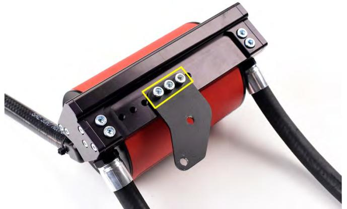
23. Locate the Street Series upper breather fitting and O-ring. Fit the O-ring onto the fitting as shown. Then insert the fitting on the top of the AOS.
