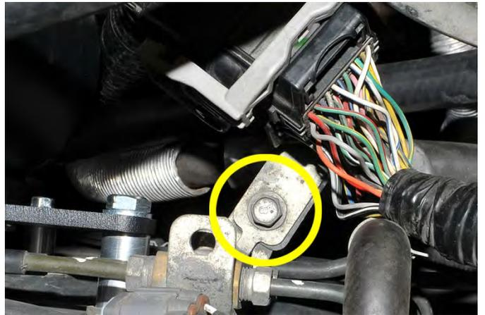
Next install the supplied harness relocation bracket using the same 10mm bolt. Do not completely tighten the bolt yet. Slide the harness onto the relocation bracket until it clips into place. Then adjust the position of the main harness for clearance and fitment. Then finish tightening the 10mm bolt. Finally reroute the primary O2 sensor wire behind the AOS and place it back into its factory support bracket. Plug the gray O2 sensor wires together.
