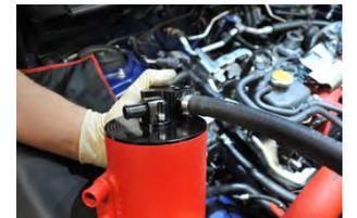
20. Install the 1/2" drain hose onto the AOS drain port fitting. Secure with a zip tie and trim the excess off.
