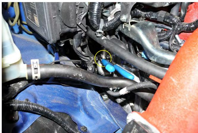
27. To minimize coolant loss, pinch off the lower coolant hose that connects the turbo to the cylinder head using hose clamping pliers.
