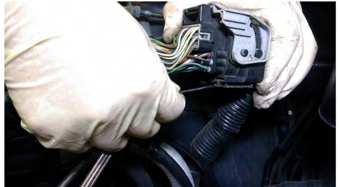
Remove the OEM electrical tape at the primary O2 sensor / main harness connection in order to add additional slack in the wiring.
