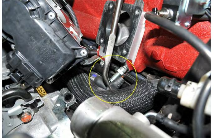
15. Install the supplied 3/8" hose on to the existing PCV nipple under the throttle body. Secure the hose with a zip tie and trim the excess off the zip tie. Leave the remaining hose free for use later in the install.
