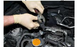
29. Using pliers remove the OEM upper coolant expansion tank hose clamp. Pull the OEM expansion hose off and slide the new IAG AOS coolant hose on. Do this fast so that coolant loss is kept to a minimum. Then using pliers pinch and slide the new supplied pinch clamp over the expansion tank port barb to secure the line.
