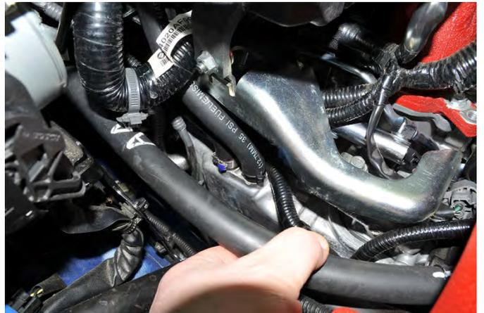
Next route the remaining portion of the hose under the intercooler bracket and alongside the 5/8” breather hose. The line will then lead up to the upper AOS port. Make sure the line is free of kinks or any obstructions. Trim the line to fit and secure it with a zip tie trimming off the excess.
