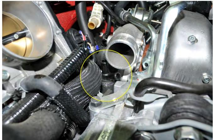
13. Using a 10mm socket, remove the (4) 10mm bolts that secure the throttle body to the intake manifold. If the throttle body is stuck, gently tap around the sides with a rubber mallet to break the throttle body free. Do not lose or damage the OEM Throttle-body gasket as it is reused.
