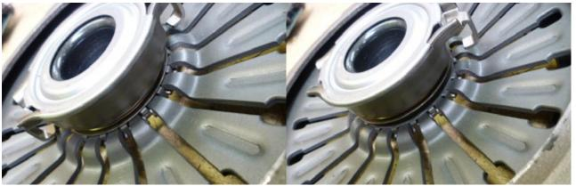
2. To remove the bearing from the cover a wedge will need to be used between the bearing and the bearing locating collar (a screwdriver can be used for this). Carefully twist the wedge so the bearing is removed on a slight angle. Removing the bearing on this angle will assist in the snap ring becoming dislodged from the locating grove.
