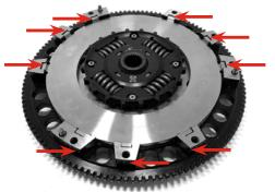
4) Install the top friction disc on the intermediate plate. Ensure on the sprung version that the outer ring is facing upward to mate correctly to the driving teeth on the bottom disc.
