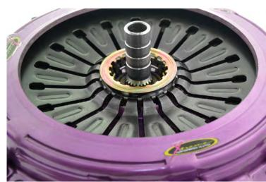
7) Slowly and evenly tighten the pressure plate bolts. The final pass should torque the bolts up to 32Nm.
