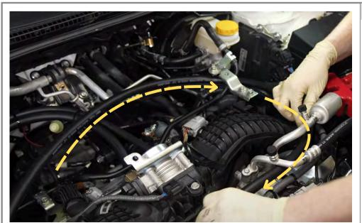
Locate the 55.5" hose and route the 45° fitting down to front of intake manifold.
