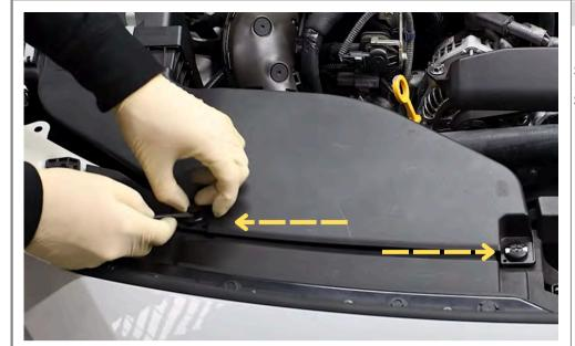
Remove the clips with a pocket screwdriver and remove the air snorkel.
