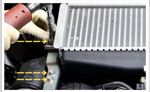
On the passenger side reinstall the three 12mm bracket bolts and tighten.
