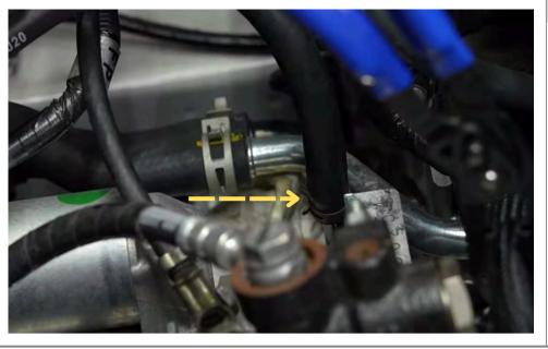
Install supplied clamp to AOS coolant hose and attach to OEM port.
