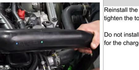
Step 63 Reinstall the charge pipe and tighten the top clamp.
