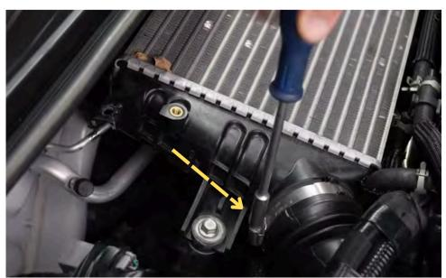
Step 9 Loosen the clamp and remove charge pipe.
