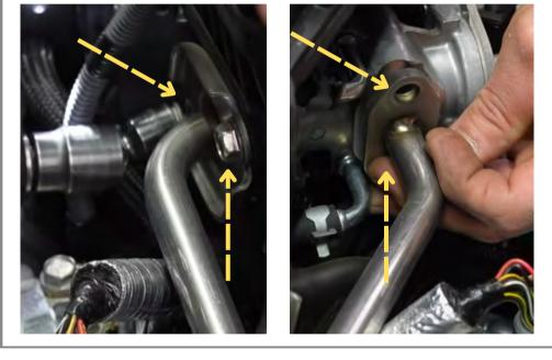
Remove the four 12mm bolts that secure the EGR pipe.
