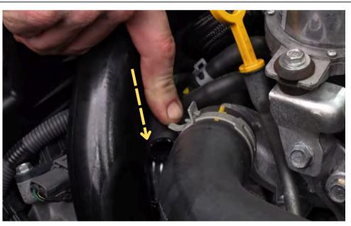
Step 65 Route fitting under charge pipe and down towards the PCV fitting.
