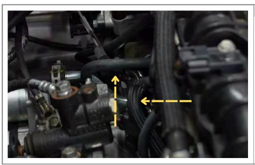
Step 36 Remove the clamps from the coolant lines from step 32.
