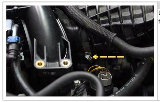
Step 12 Loosen the clamp on the throttle body.
