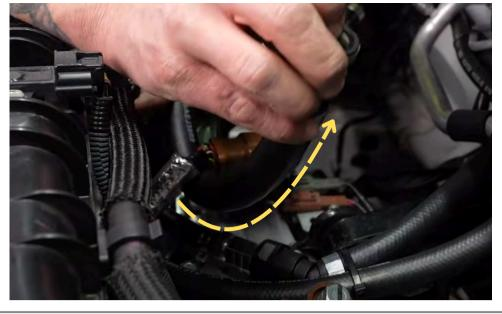
Route hose under wiring harness shown in step 57 and up to the AOS.
