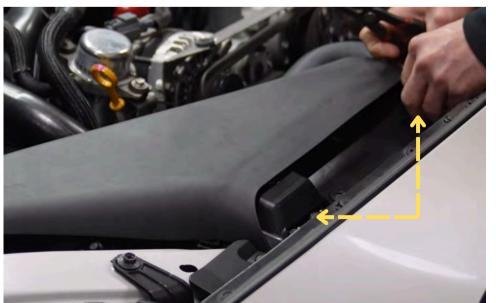
Step 3 Remove the air intake duct by removing the two front clips.
