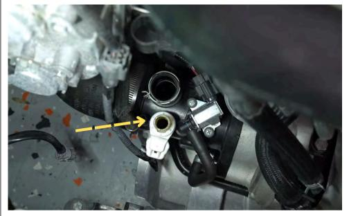
Install the PCV connector back onto the turbo inlet.
