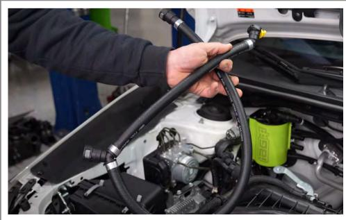
Step 42 Apply a small amount of lube to the three fittings on the Y hose.
