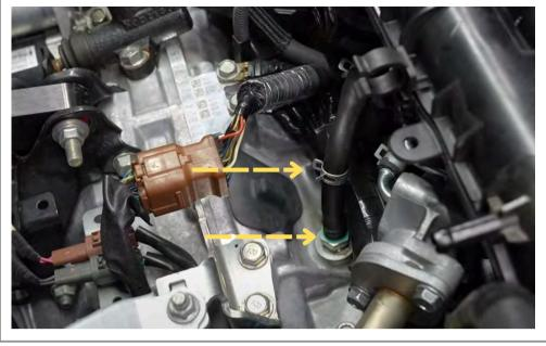
Using a pair of needle nose pliers to loosen the clamp and disconnect the hose going to the OEM PCV valve.
