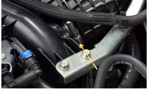
Using a nut driver, tighten the throttle body clamp.
