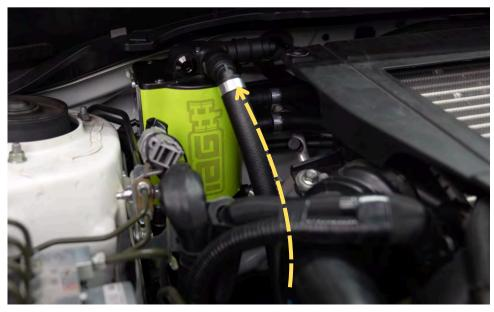
Step 70 Secure hose using a zip tie on passenger side under charge pipe.
