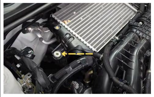
Step 11 Remove the intercooler bolt on the passenger side with a 12mm socket.
