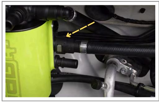
Step 45 Install fitting to middle port on AOS can.
