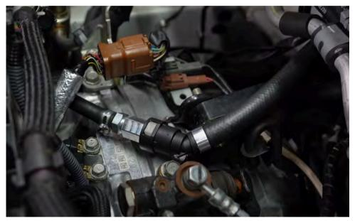
Step 41 Install the 30 degree fitting to the breather fitting.
