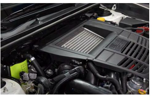
Step 73 Reinstall the plastic engine cover.
