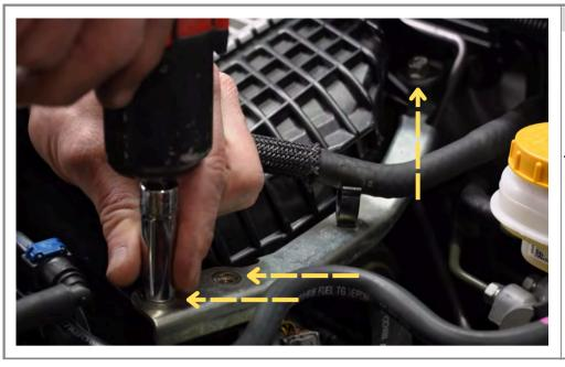
Remove the three intercooler bolts on drivers side with a 12mm socket.
