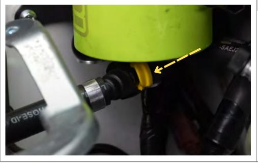
Connect drain hose on the passenger side to the bottom of the AOS can.
