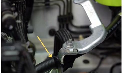
Using a zip tie secure the drain line to bracket on passenger side.
