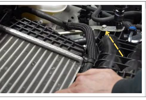
Step 61 Reinstall the intercooler and brackets back onto the engine.
