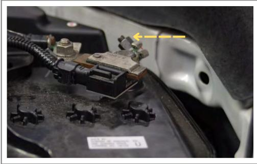
Using a 10mm wrench, remove the negative battery terminal.
