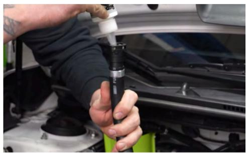
Step 56 Apply a small amount of lube to both vent hose fittings.
