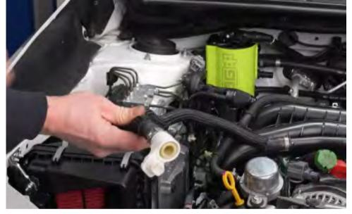
Locate the hose and connector that goes to the turbo inlet.
