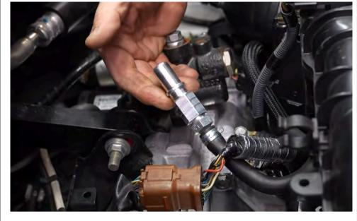
Install the new fitting into the hose that went to the OEM PCV valve.
