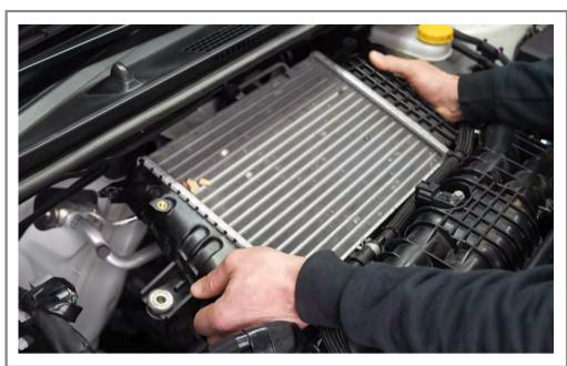
Step 13 Remove the intercooler by pulling up and away from the throttle body.
