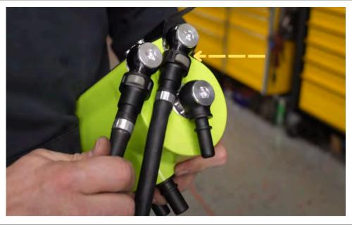
Apply a small amount of lube to fitting on the other coolant hose.
