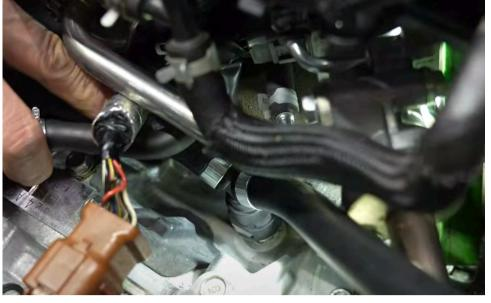
Install the Y fitting to the block breather and press down.
