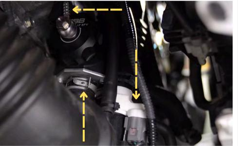
Step 68 Reinstall the clamp on BPV and vacuum line.
