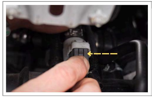
Step 6 Press tab and disconnect the electrical connector for the PCV sensor.
