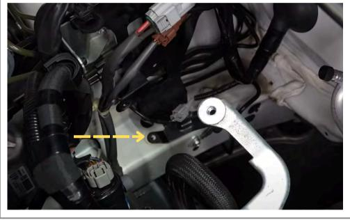
Remove the 10mm bolts which secure the ECU bracket to the strut tower.
