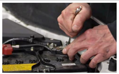
Step 74 Reattach the negative battery terminal.
