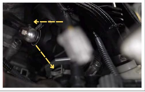
Disconnect the vacuum line that attaches to the BPV.
