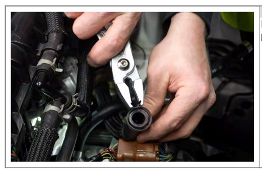
Step 55 Install clamp on OEM vent hose.
