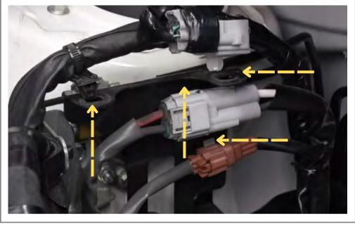
Use a pair of needle nose pliers and unclip the four electrical harnesses from the bracket.
