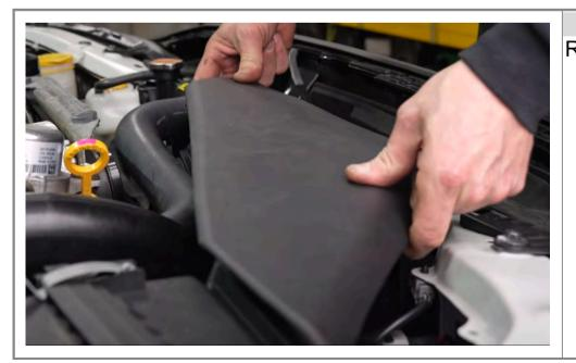
Step 72 Reinstall the intake duct.
