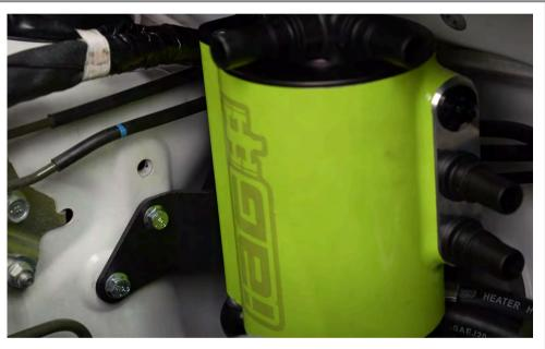
Step 29 Attach the AOS bracket to the strut tower and tighten 10mm bolts.
