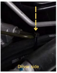
Using two zip ties secure the coolant lines to the AC hard line and brake master line.
