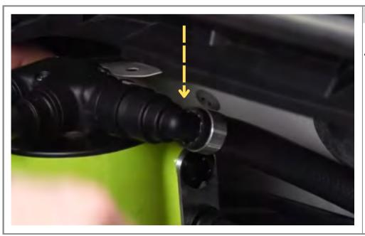
Step 39 Install 90 degree fitting to top of AOS.
