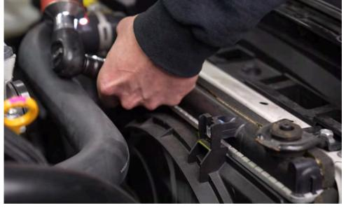
Unscrew the two bolts that secure the radiator fan.
