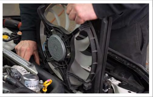
Step 71 Reinstall the radiator fan.
