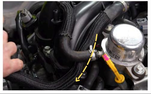
Route the vent hose under hose and behind the intake manifold.
