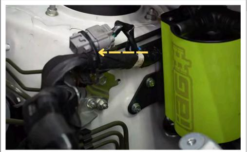
Step 30 Secure the electrical harness using a zip tie.
