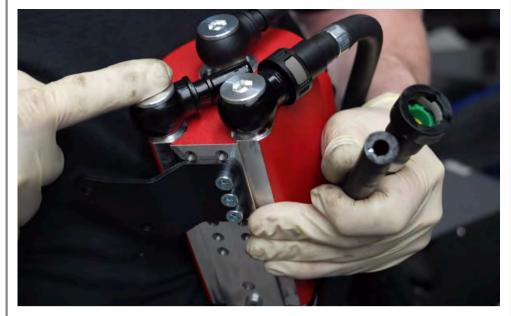
Apply a small amount of lube to fitting on the other coolant hose.
