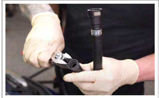
Install supplied clamp on the 90 degree fitting.
