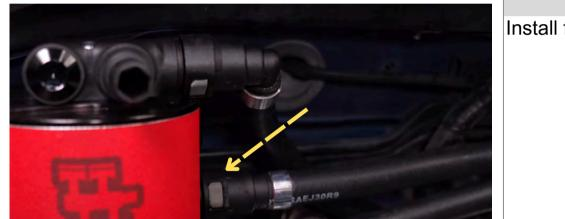
Step 63 Install fitting from hose to AOS.
