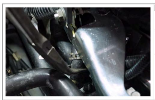
Using needle nose pliers to loosen clamp and remove hose on passenger side valve cover.
