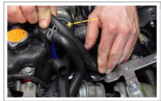
Mark where to cut the new coolant line from AOS. Use the upper expansion tank port as a reference.
