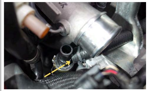
Route drain line back through the bracket and install onto breather assembly.
