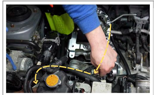
Route the AOS vent hose under the coolant line.
