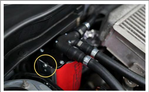
Loosen the AOS coolant breather fitting. Top off any coolant lost during installation. Start the vehicle and let it come to operating temperature. Some coolant will begin to weep from this hole. Once the air has been released tighten the bleeder fitting.
