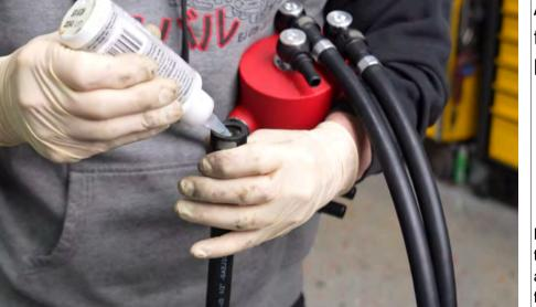
Apply a small amount of lube to the fitting on the 26 inch drain hose.
