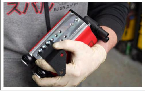
Install metal bracket to AOS and tighten until snug. Leave one hole exposed on bottom of AOS.
