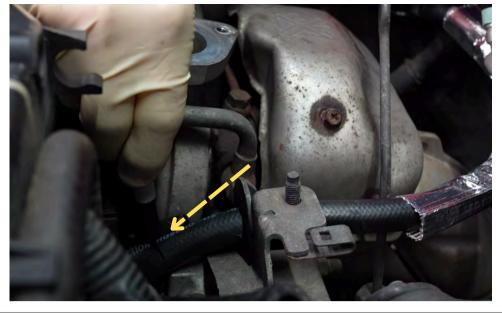
Measure the length of the drain and mark where to cut.
