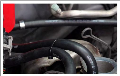
Step 38 Zip tie the two coolant lines together.
