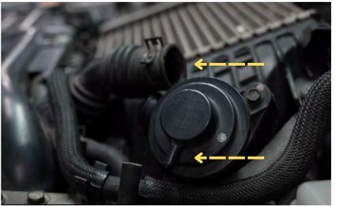
Step 3 Loosen the clamp on the two BPV hoses.
