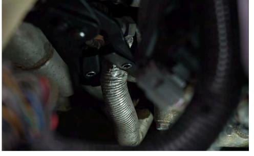
Remove the coolant hose clamp from step 28.
