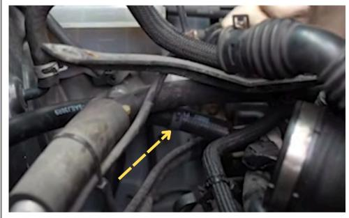
Step 54 Slide clamp on coolant line and install line onto OEM fitting.
