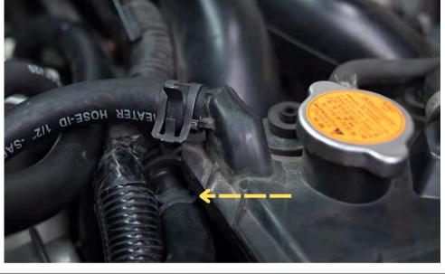
Install hose onto valve cover fitting near intake manifold.
