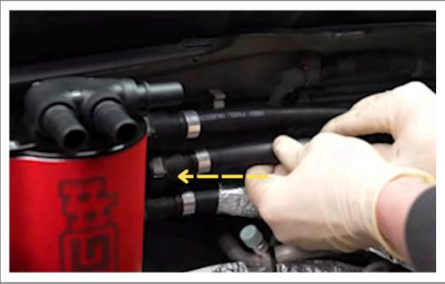
Step 57 Attach hose to middle fitting on the AOS.
