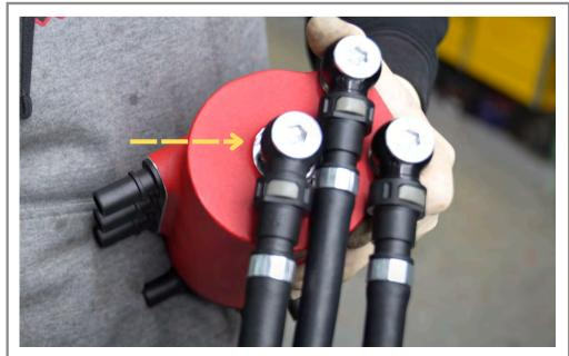
Step 23 Install drain hose to bottom of AOS can.
