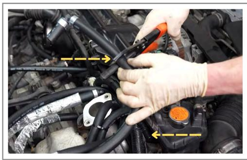
Step 85 Measure hose so it fits up to valve cover fitting.
