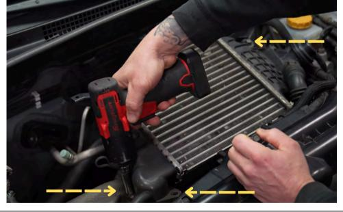
Using a 12mm socket, remove the three bolts on the intercooler.
