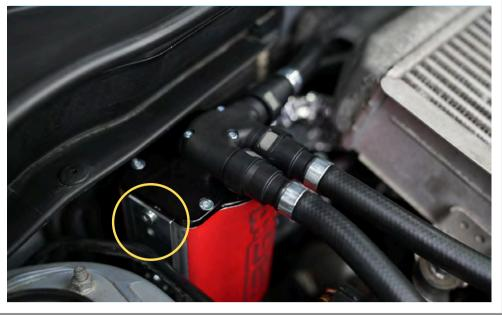
Loosen the AOS coolant breather fitting. Top off any coolant lost during installation. Start the vehicle and let it come to operating temperature. Some coolant will begin to weep from this hole. Once the air has been released tighten the bleeder fitting.
