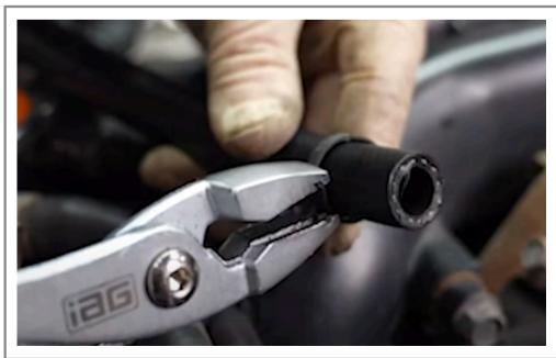
Step 71 Using a pair of pliers install the supplied clamp to the open end of the hose.
