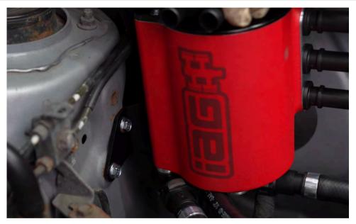
Step 25 Install the bracket and AOS onto the strut tower using a 10mm wrench.
