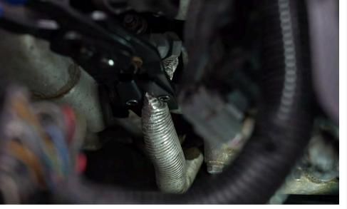
Using hose clamp pliers, clamp the turbo coolant hose.
