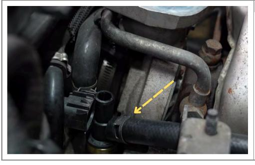
Slide clamp onto drain line and install line onto breather assembly.
