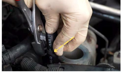
Slide clamp on coolant line and install line onto OEM fitting.
