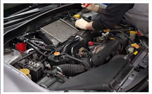
Step 89 Reinstall the top mount intercooler, BPV hoses and intercooler brackets.
