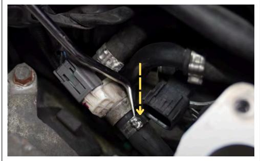
Step 8 With a pick loosen tab on the block breather hose.
