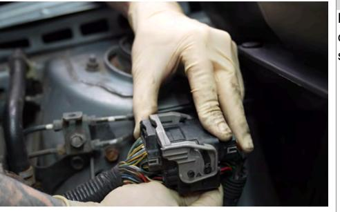
Locate the main wiring harness connector on the passenger side.
