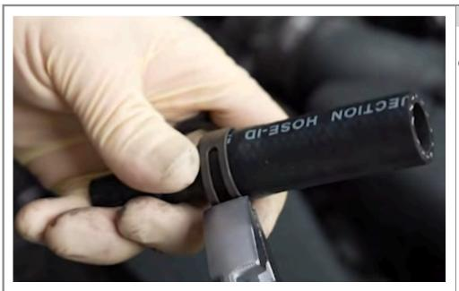
Step 14 Install fitting and two clamps onto new valve cover hose.
