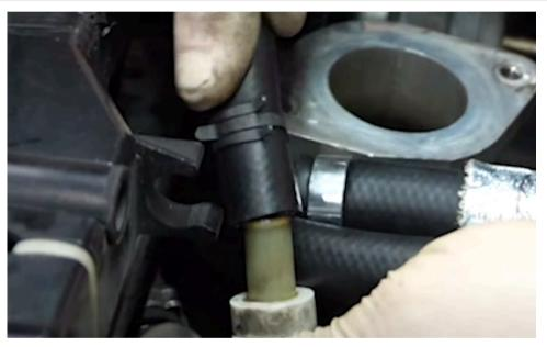
Step 82 Connect breather hose to the PCV connector and secure the clamp.
