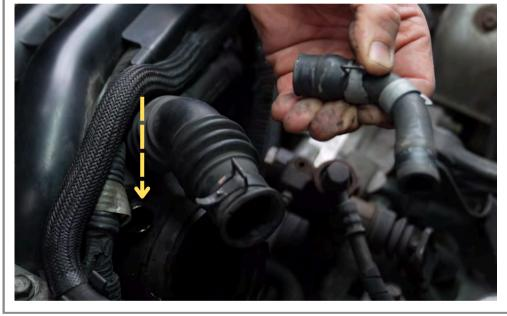
Loosen the clamp and remove the drivers side valve cover hose.
