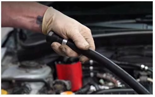
Apply a small amount of lube to the fitting on the other end.
