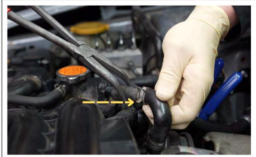
Step 29 Use a pair of needle nose pliers to loosen clamp and remove line from upper expansion tank.
