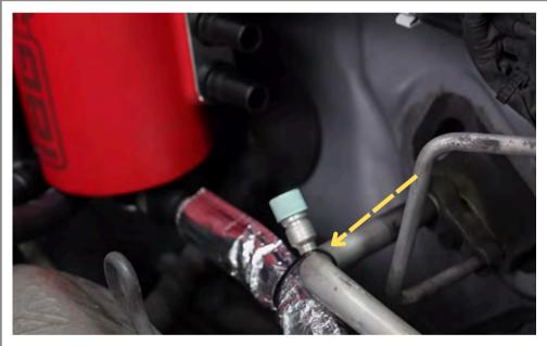
Step 46 Attach drain hose to AC hardline using a zip tie.
