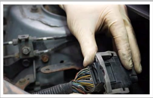
Step 19 Slide the connector off the clip that secures the connector to the bracket.
