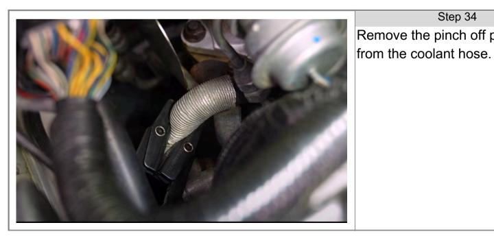
Step 34 Remove the pinch off pliers
