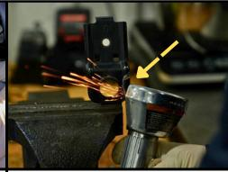
**Step 2:** With the Radiator Stay removed from the vehicle, use a Cut-Off Wheel and Grinder to remove the marked area. Once enough material has been removed, sand the Stay until smooth and reinstall in vehicle.
