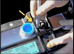
Step 1: Some vehicles may need modification to the left side radiator stay. With the Radiator installed in the vehicle, note any interference between the Stay and Radiator Cap. Mark interfering area with a sharpie or paint marker.
