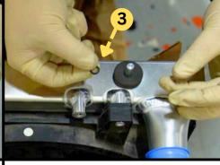
**Step 2:** Install the O-Ring over top of the Radiator Spacer to retain the Spacer to the Locating Pins.
