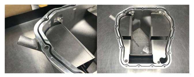
Figure 4 - O-ring Seal
