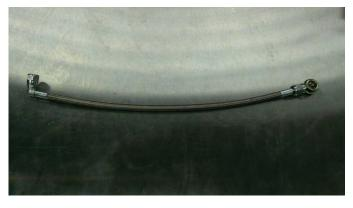
3. Using the banjo bolt that came out of the back of the head, assemble the banjo on the back oil port of the head as shown. Use a thinner washer between the head of the banjo bolt and the banjo. Then use the thicker washer between the banjo and the engine. This is the only place to use a thick washer. Torque the banjo bolt to 24  $^{\rm ft}/_{\rm lbs}$ .
