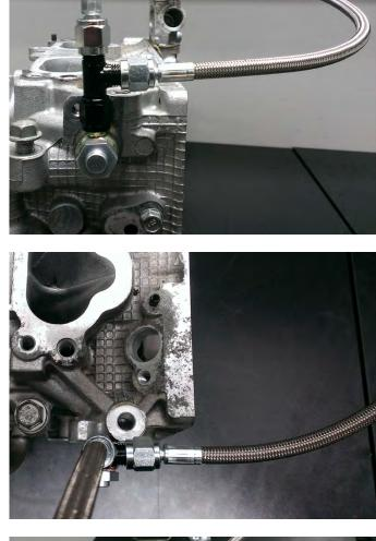
4. Install a 12mm banjo fitting on the AVCS port and point the male fitting away from the cylinder head. Run the braided line that comes out of the side of the tee fitting to the banjo fitting. Tighten the line with a  $^{9}/_{16}$ " wrench. Torque the banjo bolt to 24 <sup>ft</sup>/<sub>lbs</sub>.
