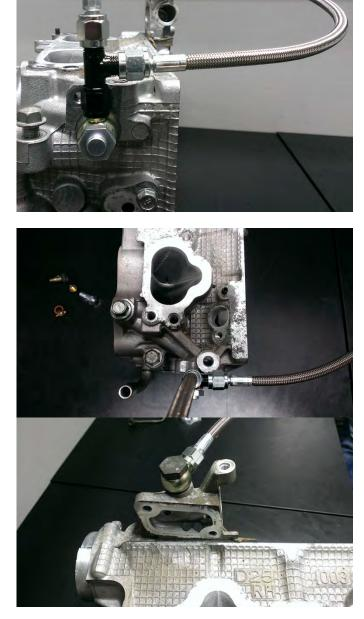
5. Install a 12mm banjo fitting on the AVCS port and point the male fitting away from the cylinder head. Run the braided line that comes out of the side of the tee fitting to the banjo fitting. Tighten the line with a  $^{9}/_{16}$ " wrench. Torque the banjo bolt to 24 <sup>ft</sup>/<sub>lbs</sub>.
