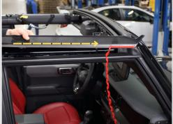
Step 6/10: Front deflector Once the rear is in line with the channel Starting from the rear of the deflector remove 75% of the tape backing
