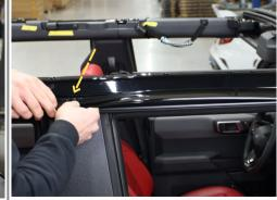
Step 8/10: Install the rear of the front deflector by bending the deflector (not letting tape touch) and click into front of rear deflector
