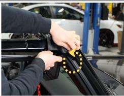
Step 7/10: Place front deflector under weather stripping. Do not let tape touch the paint.
