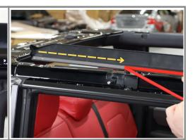
Step 3/10: Before install make sure rear of deflector fits in this channel
