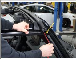
Step 9/10: Remove the rest of the tape backing and press down thoroughly to adhere along front deflector
