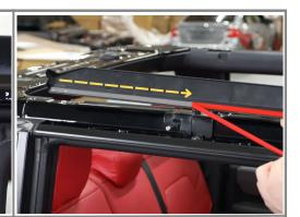
Step 3/10: Before install make sure rear of deflector fits in this channel.
