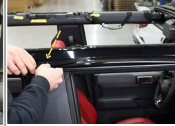
Step 8/10: Install the rear of the front deflector by bending the deflector (not letting tape touch) and click into front of rear deflector.
