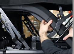
**Step 6/7:** Install the lower D-pillar cover and press down thoroughly to adhere.
