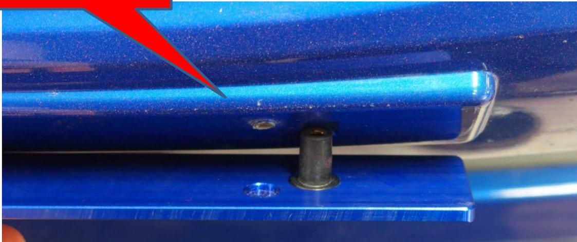
2. Press Tag Delete into the square holes in the bumper. Do not lubricate the rubber nuts.
