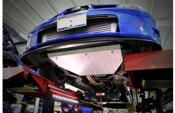
Thank you for choosing IAG Performance. The skid plate is designed to replace the factory plastic splash guard. It provides protection to the underside of the engine.
