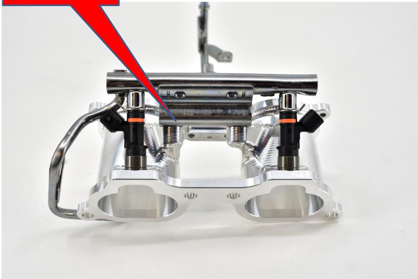
7. Install the OEM intake manifold hardware using the factory torque specifications which is 6.1 ft/lbs.
