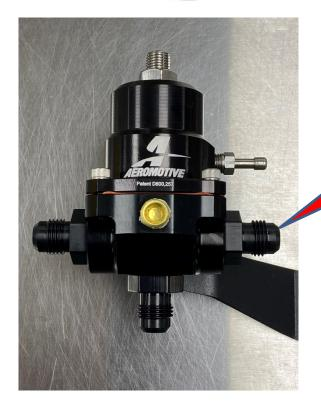
All 3 Fuel Fittings (-6 ORB to -6 AN) should be already installed, if not, install now with lube and torque to 16 ft/lbs. If used, install your Fuel Pressure Sensor or Gauge in the NPT port on the front now.
