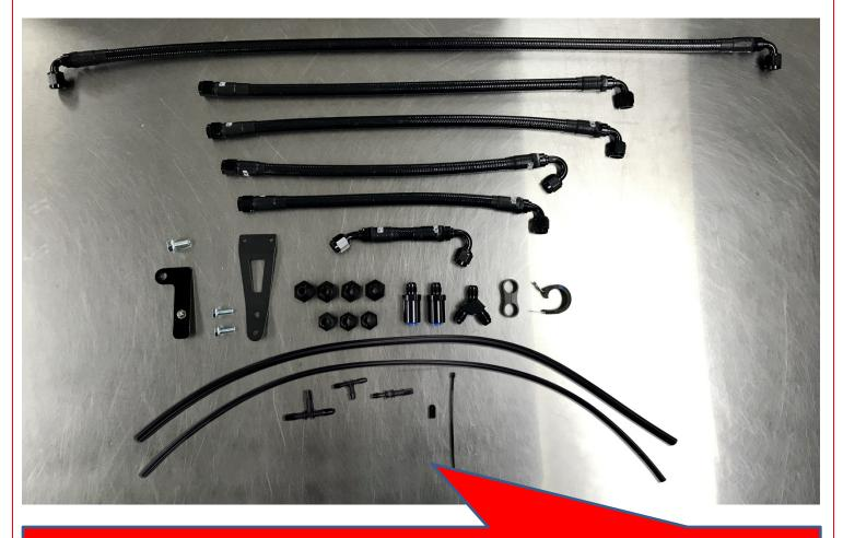
This is all of the parts laid out. Please note that each hose is identified by overall length and type of fitting used. You will see on the next page how each hose is measured, and how you can identify the proper hose. We will refer to each hose as "Hose 1, Hose 2, Hose 3, etc."
