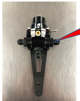
All 3 Fuel Fittings (-6 ORB to -6 AN) should be already installed, if not, install now with lube and torque to 16 ft/lbs. Install your Fuel Pressure gauge or sensor (not included) in the NPT port on the front now.
