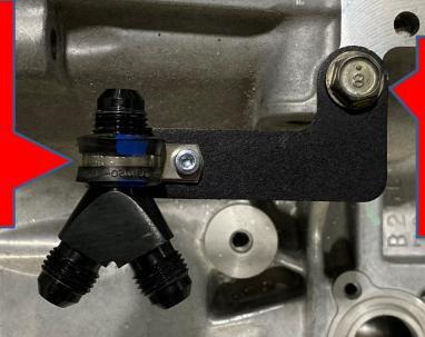
Mount the L-Bracket in the bolt hole used by the air pump bracket. Use the supplied bolt or reuse the OEM Bolt
