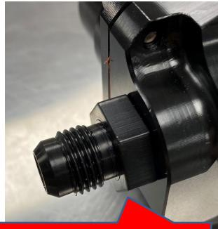
Please note that the fitting should be fully flush when installed properly. But once this fitting is flush it's fully tight.
