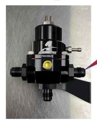
All 3 Fuel Fittings (-6 ORB to -6 AN) should be already installed, if not, install now with lube! Install your Fuel Pressure sensor in the NPT port on the front now if you are using one.
