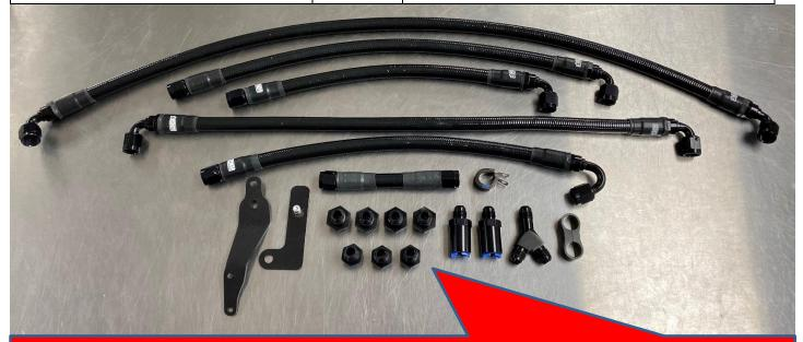
This is all the parts laid out. Please note that each hose is identified by overall length and type of fitting used. You will see on the next page how each hose is measured and how you can identify the proper hose. We will refer to each hose as "Hose 1, Hose 2, Hose 3, etc."
