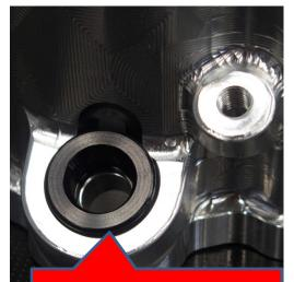
Insert lower injector adapters (with large o-rings installed and lubricated) into the TGV. They should smoothly slide in with no binding.
