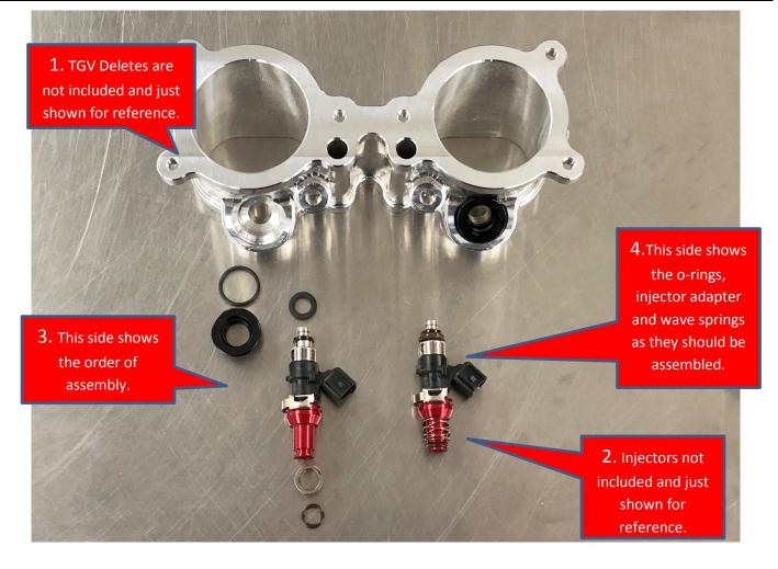
6. The ID1050x pictured below comes with the correct wave spring and orings already installed.
