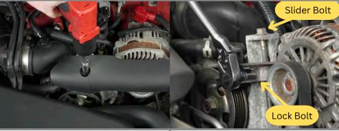
**Step 1:** Remove the 10mm bolt from the factory alternator cover.
