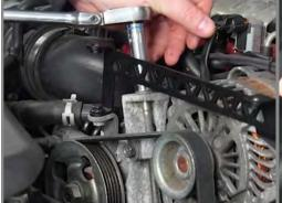
**Step 7:** Tension alternator belt to factory spec by turning Slider Bolt clockwise. Re-tighten the Lock Bolt. (25Nm)
