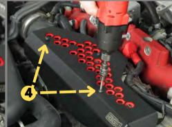
**Step 9:** Use provided 4mm Allen bolts, install Alternator Cover. Center color plate, then tighten hardware. (5Nm)
