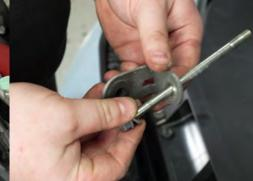
Step 4: Remove bracket from 12mm bolt.
