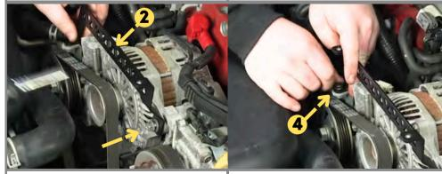
**Step 5:** Install the IAG Cover Bracket with the factory 12mm bolt. Do not tighten.
