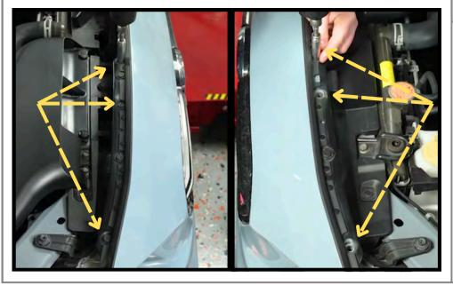
Bumper removal is required to remove factory Radiator Cover.
