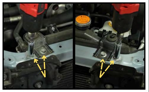
Remove the four 12mm bolts from the Radiator Stays and Radiator Support Bar.
