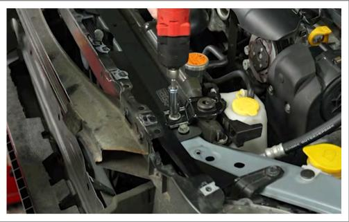
Reinstall the Radiator Stays with the factory bolts.
