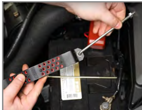
Step 5: Install the Hold Down Rods into the IAG Tie Down. Install the short rod towards the rear.
