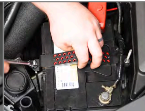
Step 6: Install the IAG Tie Down into the vehicle. Tighten down the bolts evenly to factory spec.
