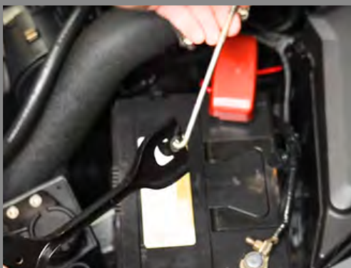
Step 4: Remove the Hold Down Rods from the factory Battery Tie Down. Replace factory nuts with provided pair.
