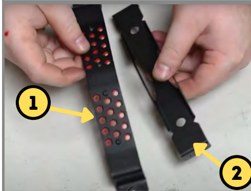
Step 2: Prepare the IAG Battery Tie Down and Tie Down Cover.
