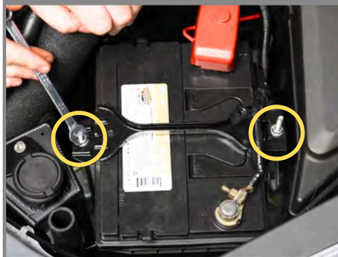
Step 3: Using a 10mm Wrench, loosen the two nuts on the factory Battery Tie Down. Remove the factory Tie Down.
