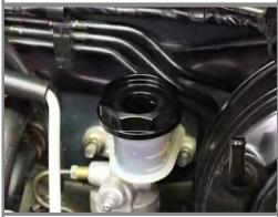
Step 5: Install the IAG Clutch Cap onto the Clutch Fluid Reservoir.
