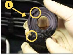
Step 3: Prepare the IAG Clutch Cap. Install factory seal onto cap. Line up notches of seal and Cap.
