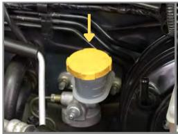
**Step 1:** Remove the factory clutch cap from the Clutch Fluid Reservoir.
