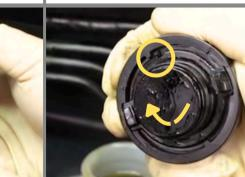
Step 4: Press factory seal into the Clutch Cap, than rotate clockwise to lock seal in place.
