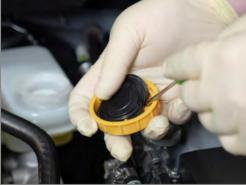
**Step 2:** Using a pocket screwdriver, remove the factory membrane from cap. Carefully pry up seal, do not damage.
