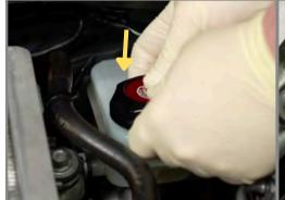
**Step 7:** Press the Decorative Cap into the Brake Fluid Cap using even pressure. Ensure the insert is fully seated.
