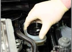
**Step 5:** Install the IAG Brake Fluid Cap onto the Brake Fluid Reservoir.
