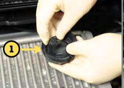
**Step 3:** Prepare IAG Brake Fluid Cap. Install factory membrane into the cap. Make sure seal is fully seated.
