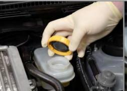
**Step 1:** Remove factory brake fluid cap from brake fluid reservoir.
