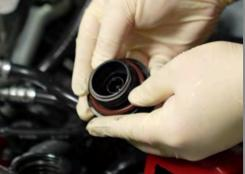
Step 3: Install the seal into the Oil Cap with the flat side facing the cap.
