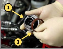
**Step 2:** Prepare the IAG Oil Cap and the provided Oil Cap Seal.
