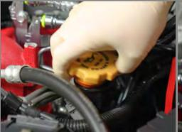
**Step 1:** Remove the factory Oil Fill Cap from the Oil Filler Neck.
