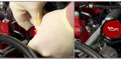
**Step 7:** Press the Decorative Cap into the Oil Cap using even pressure. Ensure the insert is fully seated.
