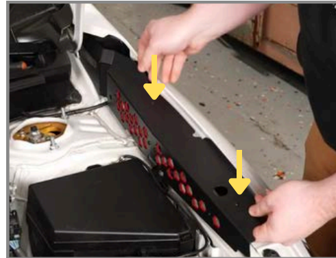
Step 7: Install the IAG Fender Shroud onto the Fender. Align the Rivet-nuts with the existing Push Clip holes.
