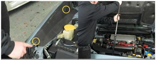
**Step 1:** Using a small pry tool, remove the push clips from the factory fender cover. Remove the fender cover.
