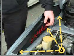
**Step 8:** Using three long 2.5mm Allen bolts, install Shroud onto fender. Apply pressure to Shroud and tighten. (5Nm)
