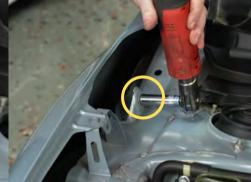
**Step 4:** Using a 12mm wrench, remove the hood strut ball.
