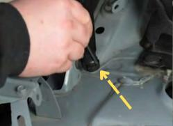
**Step 3:** Using a pocket screwdriver, pry the hood strut clip up. Remove the hood strut from the ball, and set strut aside.
