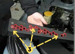
**Step 7:** Using three short 2.5mm Allen bolts, install Color Plate to the Shroud. Center the plate then tighten. (5Nm)
