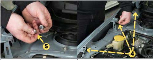
**Step 5:** Install the provided Strut Spacer onto the hood strut ball, and reinstall.
