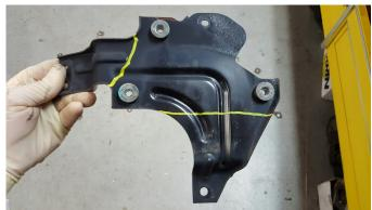
6. Using a reciprocating saw or chop saw, modify the bracket as shown.
