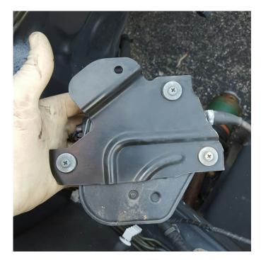
8. Using the OEM 10mm screws reattach the cruise control bracket to the strut tower to its new location as shown.
