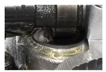
8. Remove the Pre-Oiler and adapter fitting, re-install factory switch and adapter. Reapply cam lube to the lobes and lifters to replace what may have washed off.
