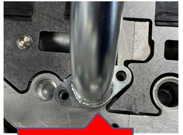
**9.** Line the Oil Pickup Flange up with the OEM mounting holes.
