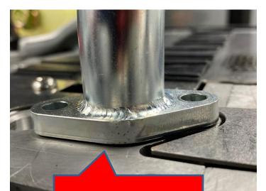
Make sure the flange is sitting flush on the block before installing the hardware.
