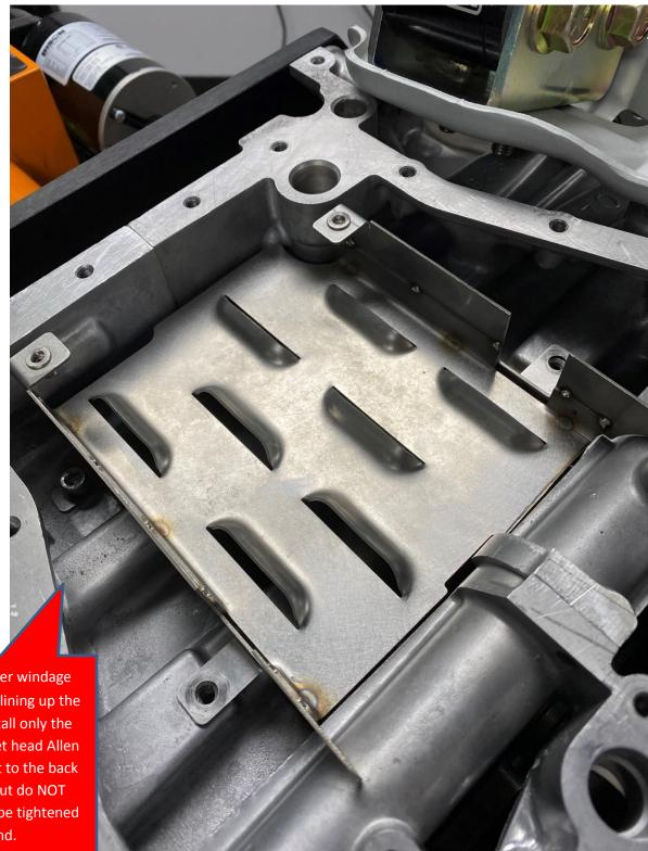
3. Place the upper windage tray in the engine lining up the 3 bolt holes. Install only the M6 x 10mm Socket head Allen in the hole closest to the back of the engine, but do NOT tighten. This will be tightened at the end.
