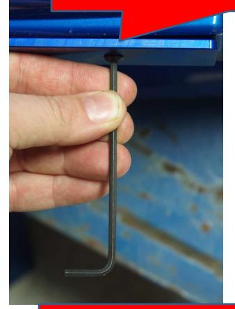
5. If the screws are tightened properly, you should not be able to pull the Tag Delete off the bumper without excessive force.
