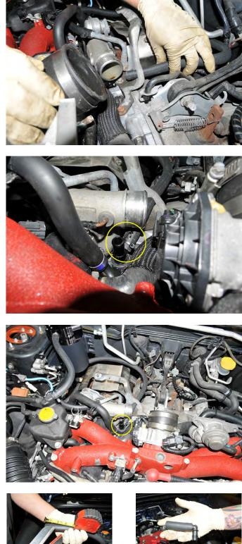
36. Locate the 5/8" breather hose and the plastic 90° fitting included with the AOS kit. Cut 3" off the breather hose. Slide the 3" length of breather hose onto one side of the 90° fitting, then slide the other side of the 3" breather hose onto the 5/8" port on the plastic drain fitting.
