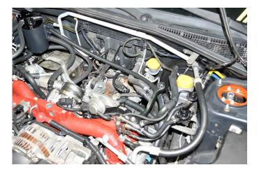
39. Route the remaining length of hose to the passenger side where the AOS located as shown. Trim the hose to fit the center port on the AOS. Then install the hose onto the port and secure it with a zip tie.
