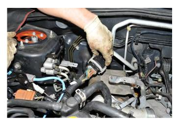
21. \* 2007 STI Only - Remove main wiring harness bracket using 10mm socket and ratchet, it is held on by (2) 10mm bolts located on the passenger side strut tower.
