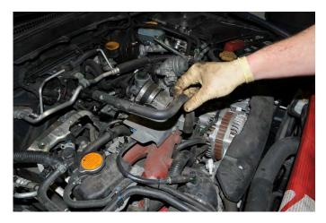
11. Using the supplied 5/8" vinyl cap, cover the hole in the inlet and secure it with a zip tie. Trim the excess of the zip tie with snips or scissors.
