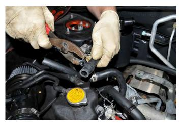
33. Using pliers remove the OEM upper coolant expansion tank hose clamp. Pull the OEM expansion hose off and slide the new IAG AOS coolant hose on. Do this fast so that coolant loss is kept to a minimum. Then using pliers pinch and slide the new supplied pinch clamp over the expansion tank port barb to secure the line.
