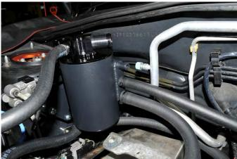
40. Using the remaining length of  $\frac{1}{2}$ " hose, route it over the top of the power steering lines and over top of the injector cover bracket. Finally slide it onto the passenger side valve cover breather port and secure it with a zip tie and trim the excess off.
