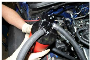
23. Next install the (2) AOS coolant lines onto the AOS (Lines come pre-assembled). Thread them on by hand and tighten using 7/8'' open end wrench.
