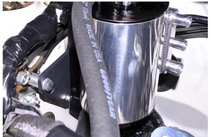
31. To minimize coolant loss, pinch off the coolant hose that connects the turbo to the engine coolant port and the lower coolant hose that connects to the EGR tube using hose clamping pliers.
