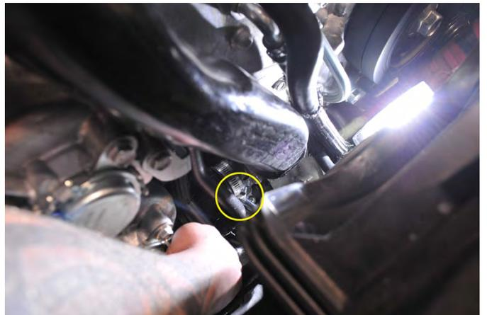
6. Using a flat head screw driver or 8mm socket and ratchet loosen the hose clamp that holds the boost pipe to the top mount intercooler. Remove the boost pipe from the vehicle by first pulling it free from the blow off valve. Then remove the pipe from the intercooler. If the rubber insert comes out reinsert it back into the pipe.
