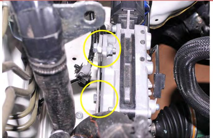
24. Next install the (2) AOS coolant lines onto the AOS (Lines come pre-assembled). \*\*The short line of the two attaches to the bottom of the AOS. Thread them on by hand and tighten using  $\frac{3}{8}$ " open end wrench.
