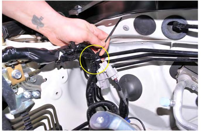
23. Locate the supplied (2) 6mm x 15mm bolts, (2) 6mm flat washers and the original (2) nuts that secured the ECU to the ECU bracket. Next using a 10mm socket, 3" extension, ratchet and 10mm wrench attach the ECU to the relocation bracket as shown. (Bolt head and washer on the bracket side, nuts on the ECU side)
