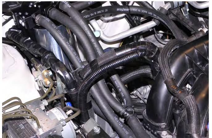
46. Route the long  $\frac{5}{8}$ " hose along the passenger side of the engine and along the front of the engine as shown.
