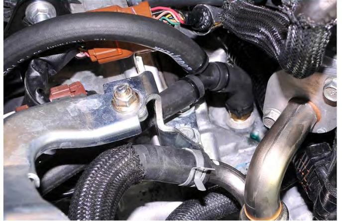
37. Locate the supplied  $\frac{5}{8}$ " cap included with the AOS kit. Attach the cap to the lowest of the three AOS ports on the can. Secure the cap with a zip tie and trim off the excess.
