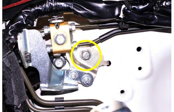
30. Install the AOS using the two holes on the strut tower shown in the picture. Guide the lower and upper coolant hose underneath the main wire harness while installing the AOS. Start the upper 13mm bolt first then start the lower 8mm bolt. Once both bolts have been slightly threaded use a 13mm and 8mm wrench to finish tightening them.
