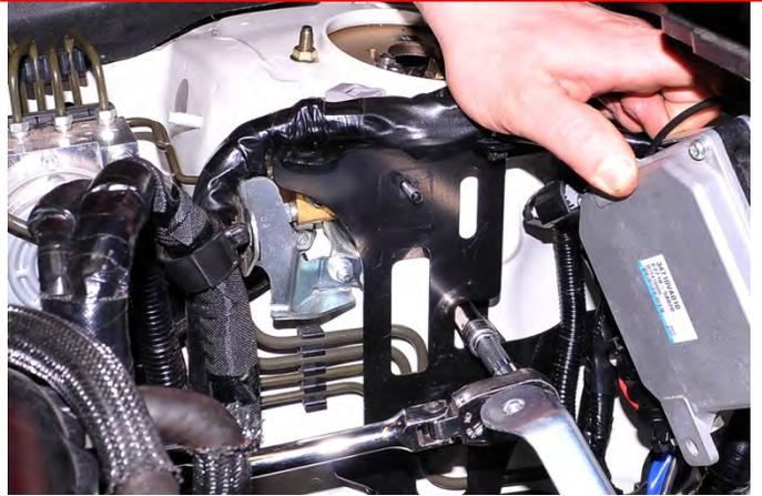
19. Pry out the small plastic plug located on the passenger side frame rail under the ground wire.
