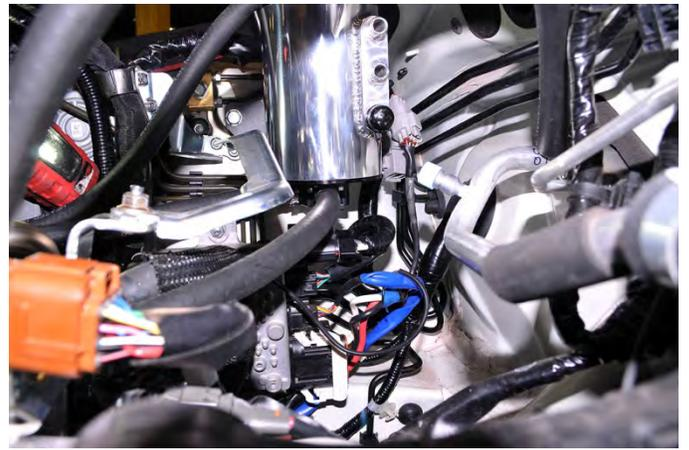
39. Locate the AOS ½" breather hose and route it to the middle AOS can port. Secure the hose the can with a zip tie. Next secure the ½" breather hose to the small AC line at the fire wall. Make sure the line is free of kinks and is not obstructed. Trim the excess off the zip ties.
