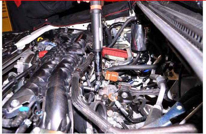
41. Locate the 1/2" AOS breather assembly. Install a zip tie loosely onto the short hose end of the breather hose assembly.
