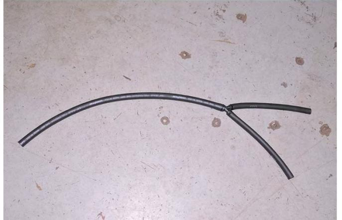
Install the shorter of the two hoses coming off the “Y” fitting onto the upper AOS breather vent hose that is closest to the strut tower.
