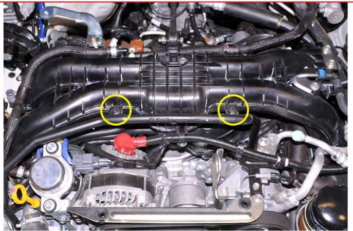
10. Using hose clamp pliers or needle nose pliers loosen the spring hose clamp on the breather pipe as shown. Then loosen the spring clamp that holds the breather to the inlet pipe. Finally remove the breather pipe from the engine retaining clip and remove the breather pipe from the engine.
