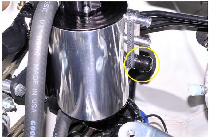
38. Locate the AOS ½" oil drain line that runs thru the intercooler support bracket. Attach the line to the lower drain port on the AOS. Make sure the line is not kinked or obstructed. Secure the line with a zip tie and trim the excess.
