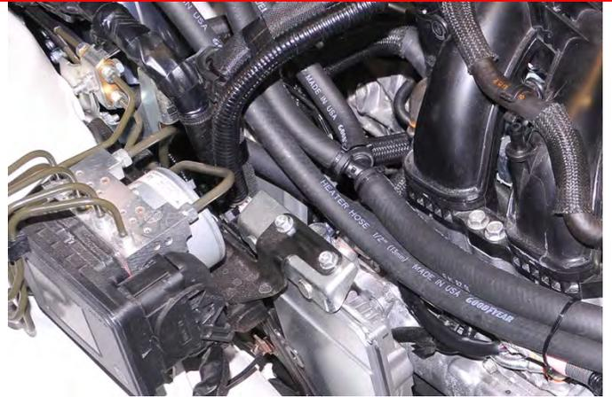
48. Reinstall the intercooler, boost pipe, intake air duct and engine cover using the OEM hardware. Reattach the negative battery terminal.
