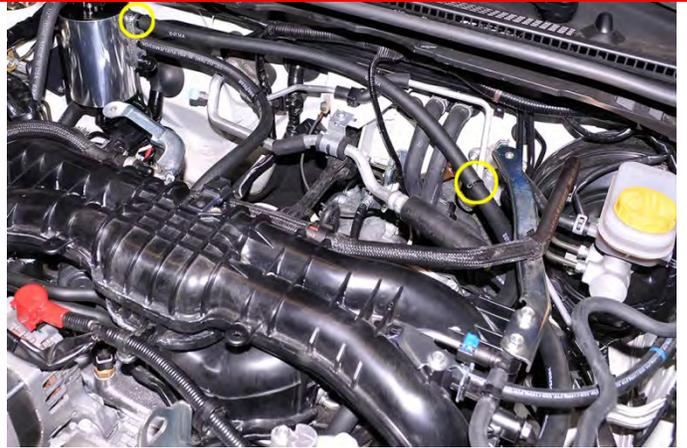
44. Locate the  $\frac{3}{8}$ " x 21" length hose and install it onto the Street Series PCV valve. Install the remaining end onto the 90°  $\frac{3}{8}$ " fitting at the intake manifold as shown. Secure both ends with zip ties and trim the excess.
