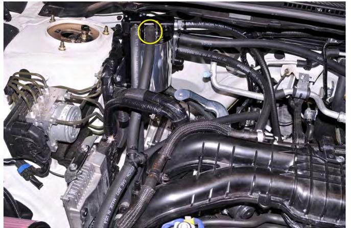
Next install the other short hose onto the remaining AOS vent port.
