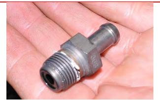
15. Next thread into the block the supplied  $\frac{3}{8}$ " NPT to  $\frac{3}{8}$ " brass barb fitting. Using the 19mm socket, ratchet and extension torque the fitting to 15ft / lbs.
