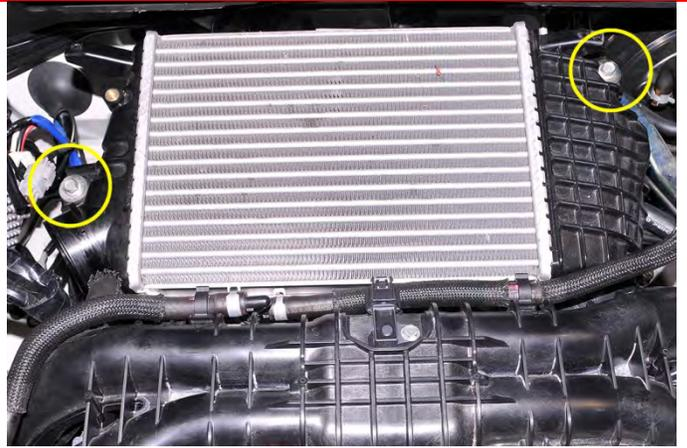
8. Loosen the hose clamp on the intercooler outlet. Then remove the intercooler from the vehicle being careful not to damage the fins or ac lines.
