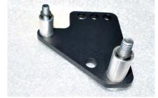
26. Install the bracket onto the AOS using the (3) small allen bolts as shown. The third hole from the bottom of the AOS should be oriented to the lowest allen bolt hole on the bracket. Tighten the three allens.
