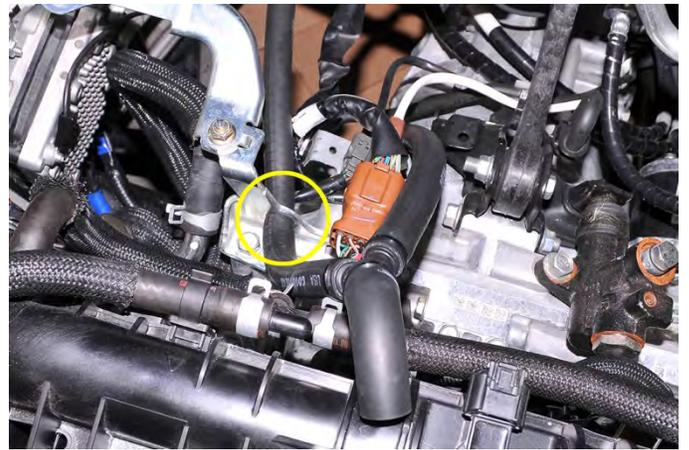
Pull the hose thru until the 90°  $\frac{5}{8}$ " hose lines up with the brass barb fitting on the engine block. Push the 90 degree  $\frac{5}{8}$ " hose onto the brass barb and secure it with a zip tie. Trim the excess off the zip tie.
