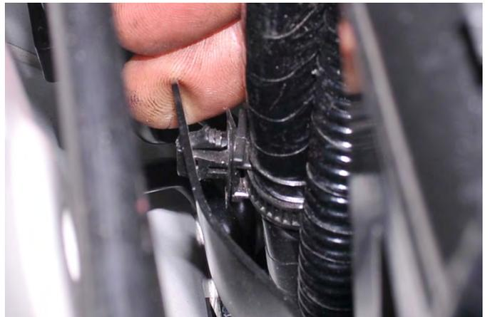
17. Using a 10mm socket, ratchet and 3" extension remove the (2) 10mm nuts that hold the ECU to the bracket. Then pull the ECU free from the bracket and place it aside in the engine bay.
