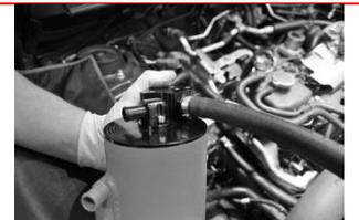
25. Assemble the AOS mounting bracket. Locate the bracket the hardware bag. Install the included flat washers on each of the bolts. Place the bolts thru the bracket as shown. Next install the included spacers. The recessed portion of the spacer faces away from the bracket. Then install the O-rings onto the bolts to secure the spacers in place.
