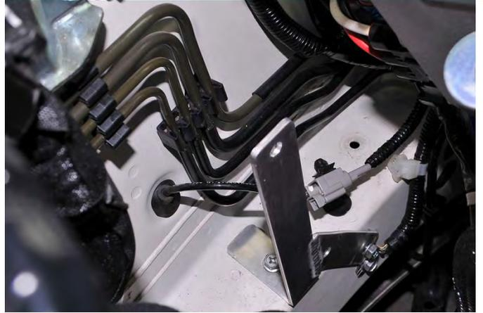
22. Using a 10mm socket and ratchet remove the 10mm bolt that secures the wiring harness onto the ECU.
