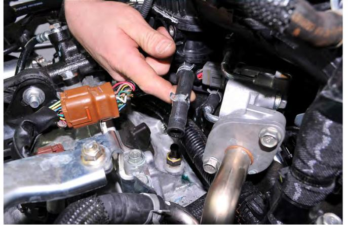
14. Using a 19mm socket, 8" extension and ratchet remove the PCV valve from the engine short block.
