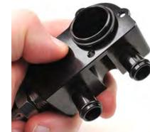
28. Clock the upper breather fitting so that it matches the picture. Locate the (3) supplied 4mm x 8 allen bolts and using a 3mm allen wrench thread the bolts thru the breather fitting into the AOS and secure the port fitting.
