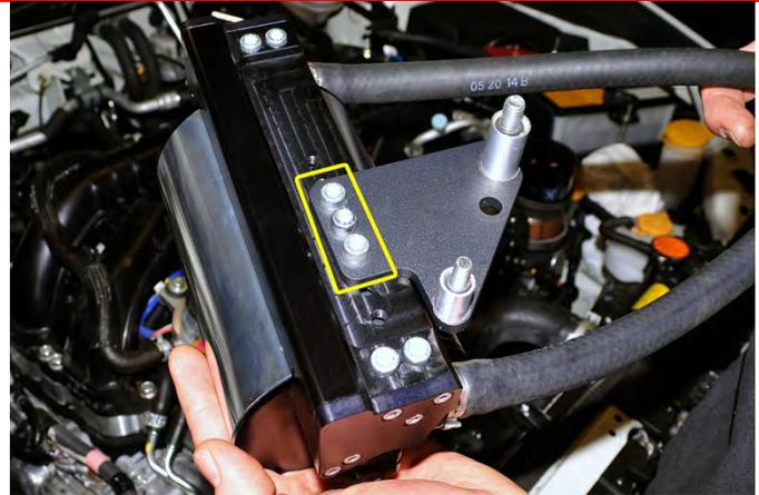
27. Locate the Street Series upper breather fitting and O-ring. Fit the O-ring onto the fitting as shown. Then insert the fitting on the top of the AOS.
