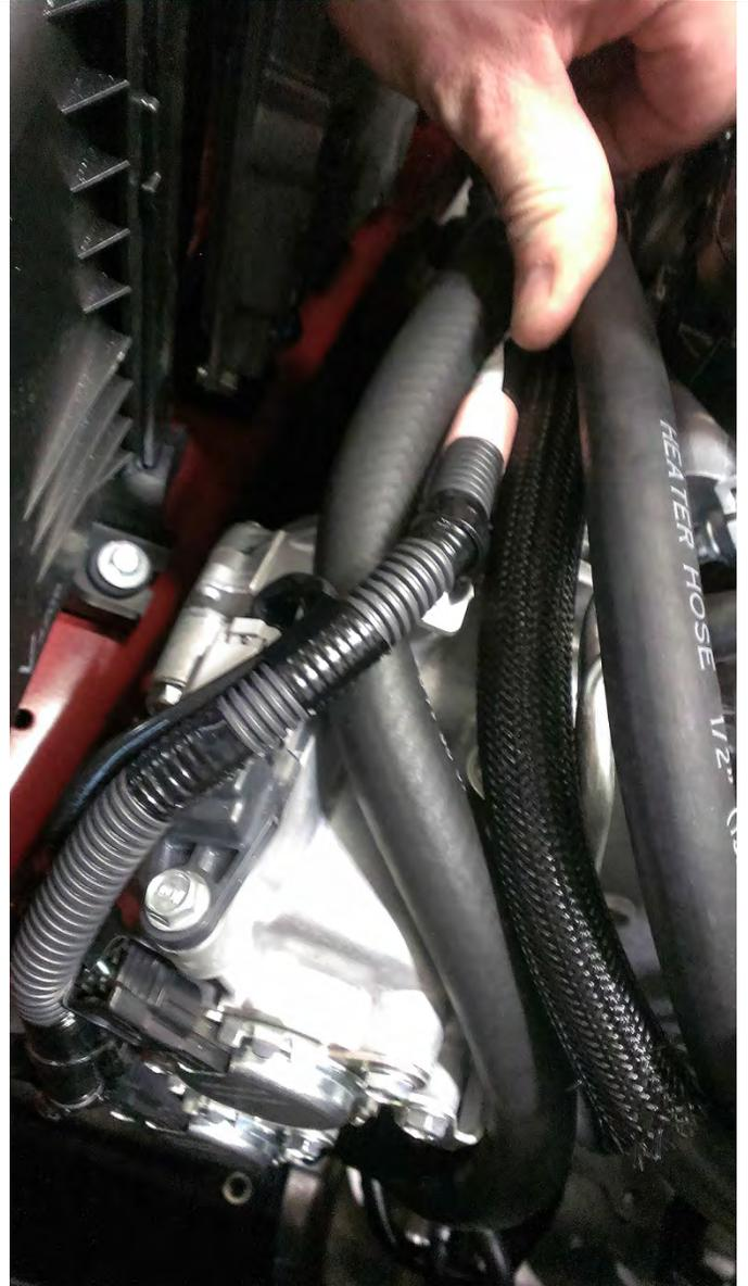
Route the hose down to the inlet port. Attach the hose to the inlet and secure it with a zip tie. Trim the excess off the zip tie.
