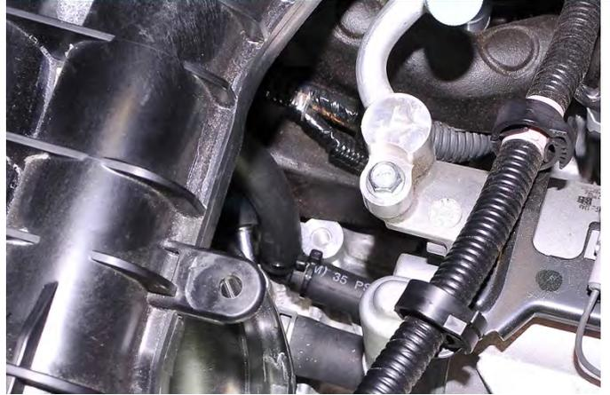
43. Route the long portion of the  $\frac{1}{2}$ " breather hose along the firewall to the top  $\frac{1}{2}$ " port on the AOS as shown. Secure the hose with a zip tie at the port and onto the small AC line at the fire wall. Trim the excess off the zip ties.
