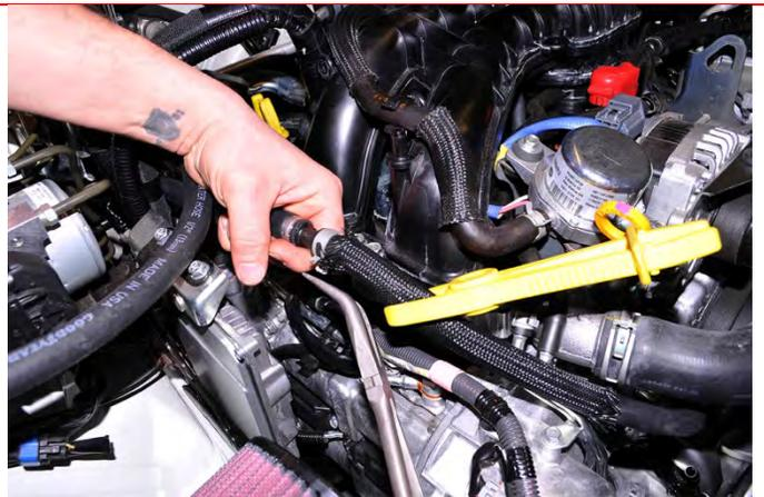
33. Slide the OEM coolant hose onto the lower AOS coolant hose straight fitting. Next using pliers and the OEM spring clamp secure the OEM hose to the fitting.
