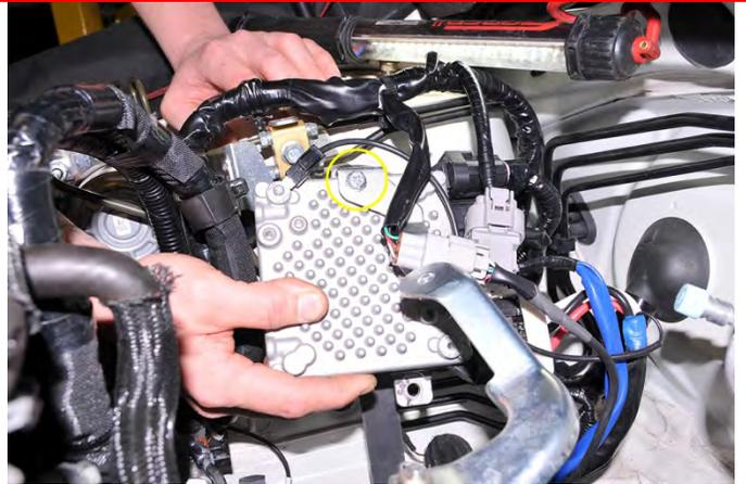
Next remove the wiring retaining clip from the bracket and remove the bracket from the vehicle.
