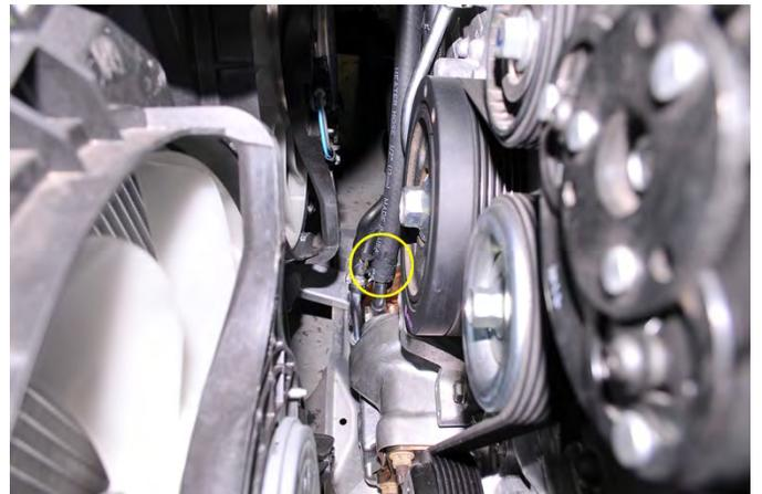
35. Remove all the hose clamping / pinching pliers.
