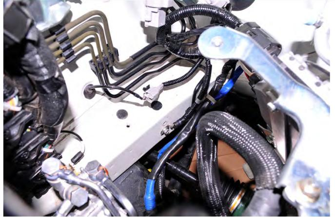
21. Locate the supplied ECU relocation bracket. Attach the bracket using the (2) 10mm bolts that held the original bracket to body of vehicle as shown. Using a 10mm socket, 8" extension and ratchet tighten the 10mm bolt on the top frame rail. Then using a 10mm socket and ratchet tighten the 10mm bolt on the side of the frame rail.
