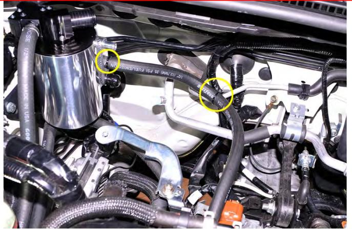
40. Reinstall the OEM EGR pipe and gasket using the (4) OEM 12mm bolts. Torque is 14ft. / lbs. \*Make sure before installing the EGR pipe that the OEM O-ring is in place on the intake manifold.
