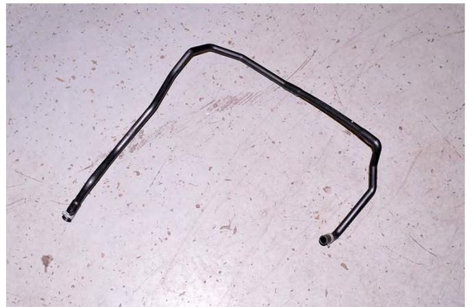
11. Using a 12mm socket, 3" extension and ratchet, remove the (4) 12mm bolts that hold the EGR pipe on the EGR valve and intake manifold. Be careful not to lose or damage the metal gasket at the EGR valve as it is reused. Remove the pipe from the vehicle.
