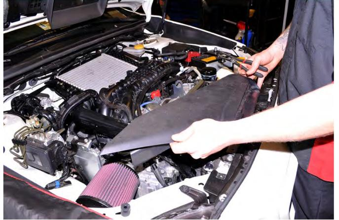
5. Next using a  $\frac{3}{8}$ " long extension, ratchet and 12mm socket remove the (2) 12mm bolts that hold the boost pipe to the turbo. Then using an 8mm socket loosen the clamp that holds the blow off valve. This can be done from above or below the car. If removing from underneath the car remove the OEM belly pan.
