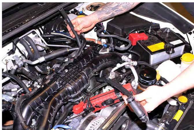
Then attach the short  $\frac{1}{2}$ " hose with the loose zip tie to the block breather port under the AC compressor as shown. Secure the short hose with the zip tie and trim the excess.
