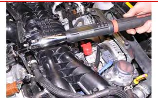
16. Remove the (4) wiring harness retaining clips from the ECU mounting bracket. Using needle nose pliers squeeze the locking tabs to free them from the bracket.
