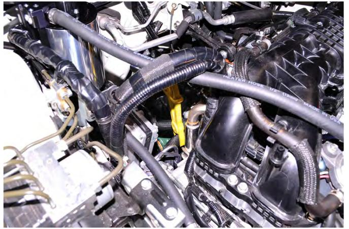
32. Using needle nose pliers remove the spring clamp at the turbo coolant port. Next loosen the spring clamp on the coolant line at the engine and rotate the hose towards the strut tower so that it can meet up with the lower AOS coolant hose.
