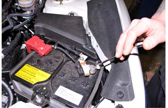
3. Using pop clip pliers remove the upper engine cover's (2) pop clips, then remove the cover from the vehicle.
