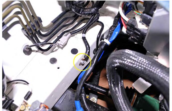
20. Relocate the ground wire to the lower frame bolt hole as shown using the OEM bolt. Tighten the bolt using a 10mm socket and ratchet.
