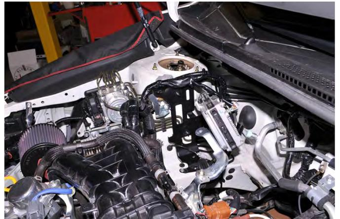
18. Remove the (2) 10mm bolts that hold the ECU bracket to the passenger side strut tower and frame rail as shown. Then remove the bracket from the vehicle.
