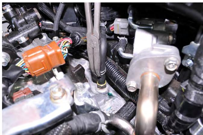
13. Next pull the PCV hose free from the PCV valve and insert the  $\frac{3}{8}$ " plastic 90° fitting into the hose. Finally using the OEM spring clamp, secure the fitting in the hose.
