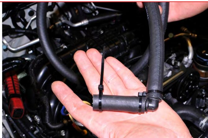
42. Route the long ½" breather assembly hose under the intake manifold towards the brake master cylinder.
