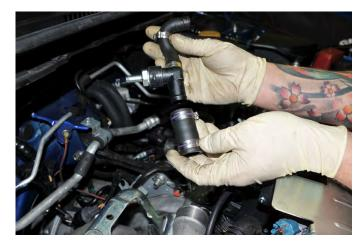
12. Slide the supplied plastic drain fitting into the  $\frac{3}{4}$ " drain hose as shown.
