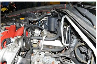
35. Locate the ½" breather line included in the AOS kit. Route one side of the line to the driver side most forward valve cover breather port. The line should pass over top the fuel injector cover bracket until it meets the valve cover port. Slide the hose onto the port and secure it with a zip tie.
