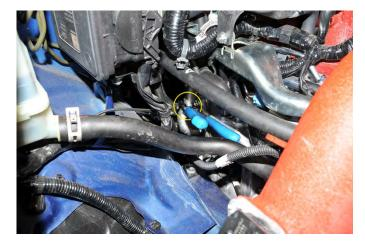
29. The IAG AOS coolant line will attach to the OEM coolant expansion tank. Trim the upper AOS coolant line to the correct length making sure when the line is routed there are not any kinks or obstructions. Once cut, using pliers pinch and slide the supplied pinch clamp onto the AOS coolant line.
