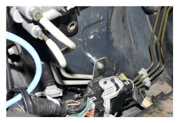
27. Install the AOS using the two holes on the strut tower shown in the picture. Start the upper 13mm bolt first then start the lower 8mm bolt. Once both bolts have been slightly threaded use a 13mm and 8mm wrench to finish tightening them.
