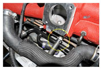
16. Re-install the throttle body to the intake manifold. Torque the (4) 10mm bolts to 6  $^{\rm lb}/_{\rm ft}$ .
