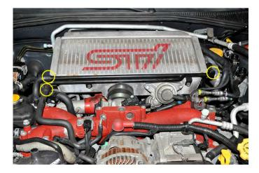
4. Using a 12mm socket, remove the intercooler mounting bolts on either side of the intercooler.
