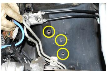
20. Next install the (2) AOS coolant lines onto the AOS (Lines come pre-assembled). Thread them on by hand and tighten using 7/8" open end wrench.
