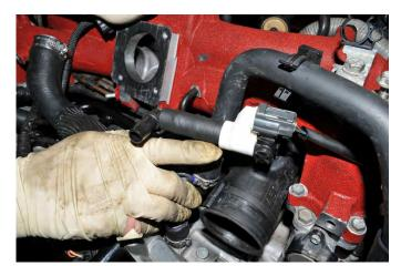
41. Install the remaining length of  $\frac{1}{2}$ " hose onto the plastic 90° fitting. Then route the remaining portion to the port on the AOS breather. Trim the excess and secure all the connections with zip ties.
