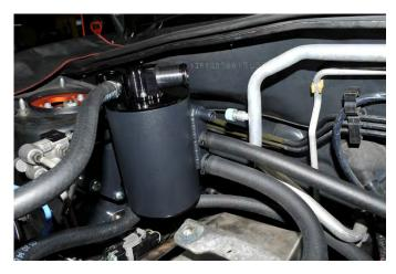
37. Using the remaining length of ½" hose, route over the top of the power steering lines and over top the injector cover bracket. Finally slide it onto the passenger side valve cover breather port and secure it with a zip tie and trim the excess off.
