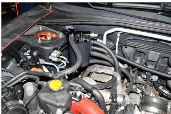
38. Route the 3/8" hose from the PCV nipple under the throttle body to the PCV located at the top breather port of the AOS. Keep the line as low as possible next to the transmission housing. Trim the hose to fit and secure with a zip tie. Trim excess off the zip tie.
