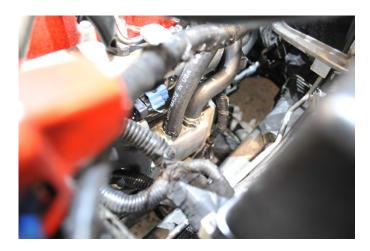
36. Route the remaining length of hose to the passenger side where the AOS located as shown. Trim the hose to fit the center port on the AOS. Then install the hose onto the port and secure it with a zip tie.
