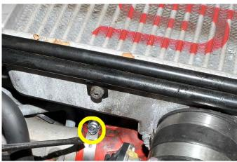
7. Using a flat head screw driver, loosen the hose clamp at the intercooler outlet silicone coupler.
