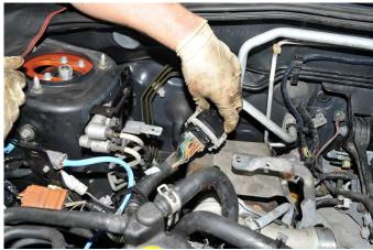
18. \* 2007 STI Only - Remove main wiring harness bracket using 10mm socket and ratchet, it is held on by (2) 10mm bolt located on the passenger side strut tower.
