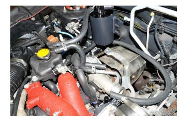
Remove the upper OEM coolant line pinch clamp and pull the OEM line off the turbocharger. Remove the OEM line from the vehicle.
