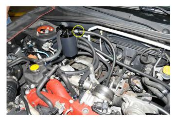
39. Insert supplied  $\frac{1}{2}$ " straight fitting into the OEM breather hose as shown. Then install the supplied  $\frac{1}{2}$ " hose onto the plastic fitting . Route the hose to the upper AOS breather fitting as shown. Trim the hose to fit and secure connections with zip ties.
