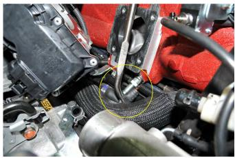
15. Install the supplied 3/8" hose on to the existing PCV nipple under the throttle body. Secure the hose with a zip tie and trim the excess off the zip tie. Leave the remaining hose free for use later in the install.
