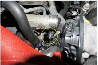
33. Locate the 5/8" breather hose and the plastic  $90^\circ$  fitting included with the AOS kit. Cut 3" off the breather hose. Slide the 3" length of breather hose onto one side of the  $90^\circ$  fitting, then slide the other side of the 3" breather hose onto the 5/8" port on the plastic drain fitting.
