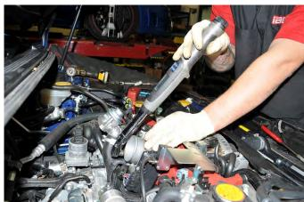
17. \* 2007 STI Only - Remove the main engine harness from its mounting bracket located on the passenger side strut tower. Using a flat head screw driver start by unclipping the harness hold down clamp. Then using a flat head screw driver pry the main harness clip outwards and lift out as shown.
