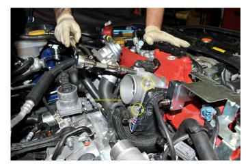
14. Remove the small pinch clamp and hose from the PCV vacuum nipple under the throttle body on the intake manifold using needle nose pliers.
