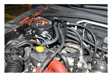
40. Locate the remaining  $\frac{1}{2}$ " hose supplied with the kit. Cut 2" off and insert it onto the supplied  $\frac{1}{2}$ " 90° degree plastic fitting. Then install the  $\frac{1}{2}$ " hose and 90 onto the white portion of the blow-by sensor.
