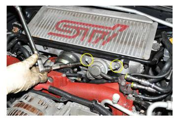
6. Using a flat head screw driver, loosen the hose clamp on the turbo discharge silicone coupler.
