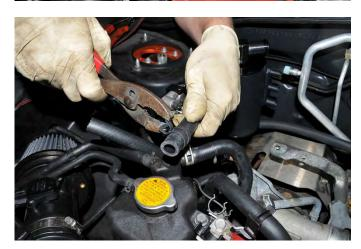
30. Using pliers remove the OEM upper coolant expansion tank hose clamp. Pull the OEM expansion hose off and slide the new IAG AOS coolant hose on. Do this fast so that coolant loss is kept to a minimum. Then using pliers pinch and slide the new supplied pinch clamp over the expansion tank port barb to secure the line.
